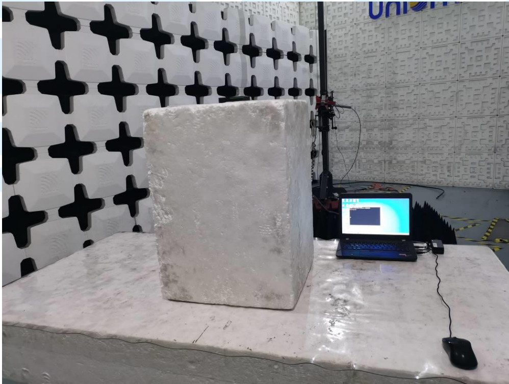
Radiated emission Test Setup (Above 1 GHz)
