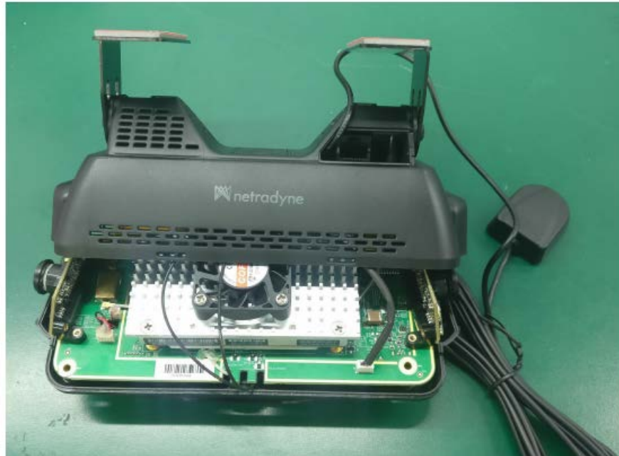
Top Cover View Main PCB connected to Power PCB (RJ-45 PCB)
