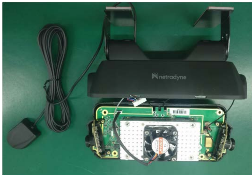
Top Cover View Main PCB disconnected to Power PCB (RJ-45 PCB)
