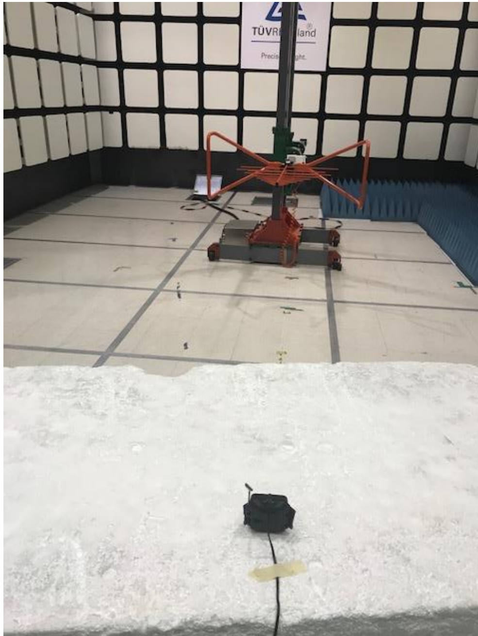
Radiated Emissions Setup 30 to 1000 MHz rear
