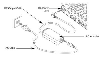
Figure 3-1 Connecting the AC Adapter
