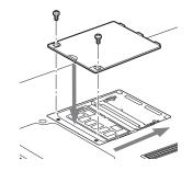
Figure 4-9. Replacing the Memory Compartment Cover
