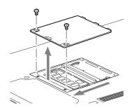
Figure 4-7. Opening the Memory Upgrade Compartment
