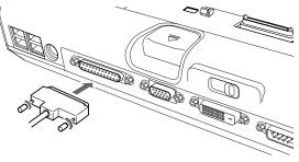
Figure 4-17. Connecting a Parallel Device to Port Replicator
