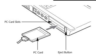
Figure 4-6. Installing/Removing PC Cards
