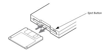
Figure 4-4.Loading/Ejecting a 3.5" Floppy Disk
