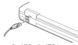
Figure 4-19. Connecting a USB Device
