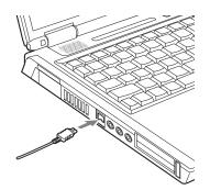
Figure 4-20. Connecting an IEEE 1394 Device
