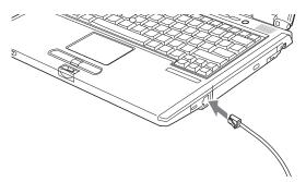
Figure 4-15. Connecting a Modem
