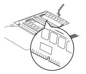
Figure 4-8. Installing a Second Memory Module
