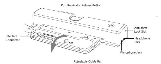
Figure 4-12. Port Replicator front panel
