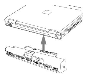
Figure 4-13. Attaching the Port Replicator
