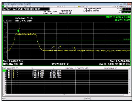
Test result: The unit does meet the FCC requirements.
