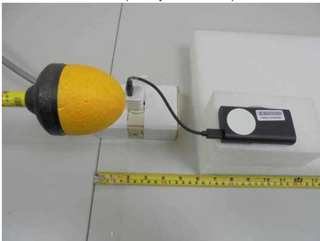
E-Field (Standby Mode - Bottom)
