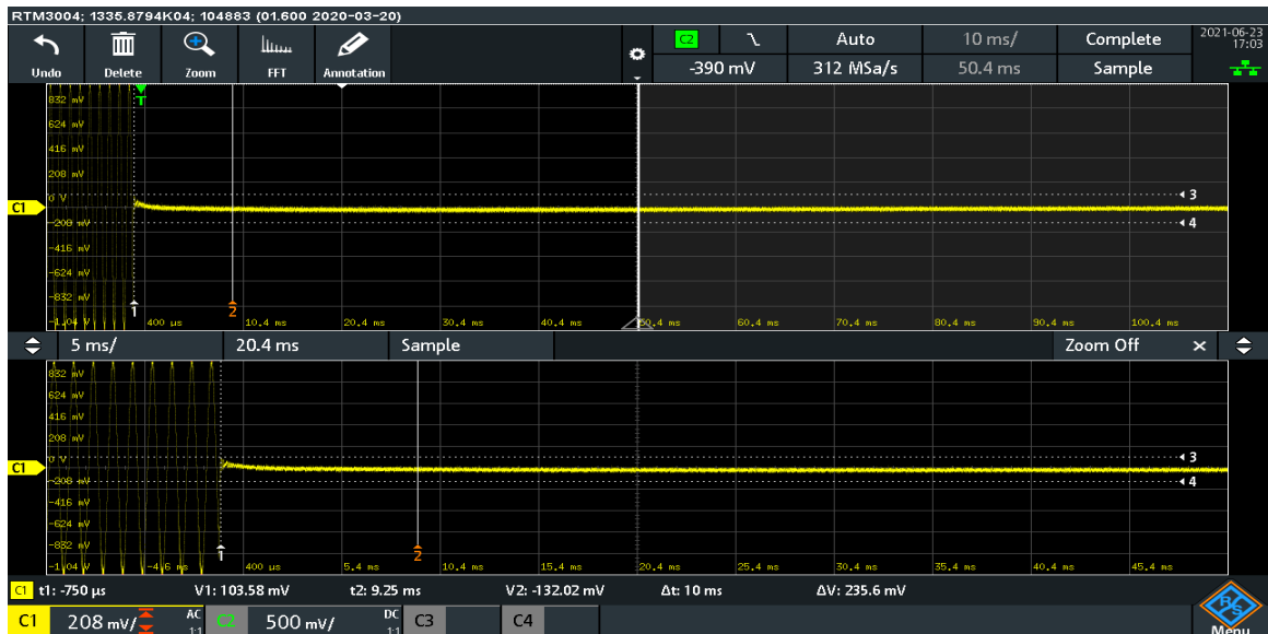
Plot 7.6.1 Transient frequency during power ON test results at low carrier frequency
