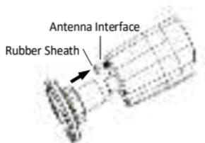
7. Rotate the antenna to the antenna interface according to clockwise direction.
