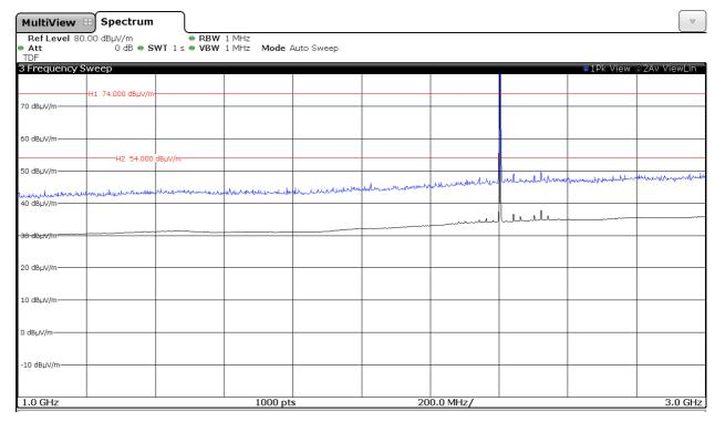
Note: The peak shown in the plot above the limit is the carrier frequency.
