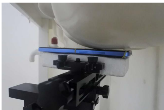
Left Cheek, Test Separation 0 mm
