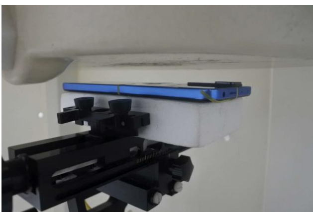
Back, Test Separation 15 mm(sensor off)
