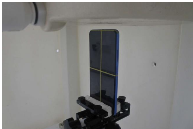
Top Side, Test Separation 10 mm
