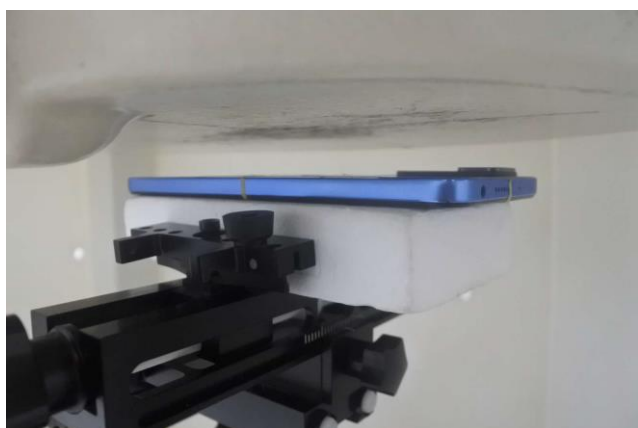
Back, Test Separation 20 mm(sensor off)
