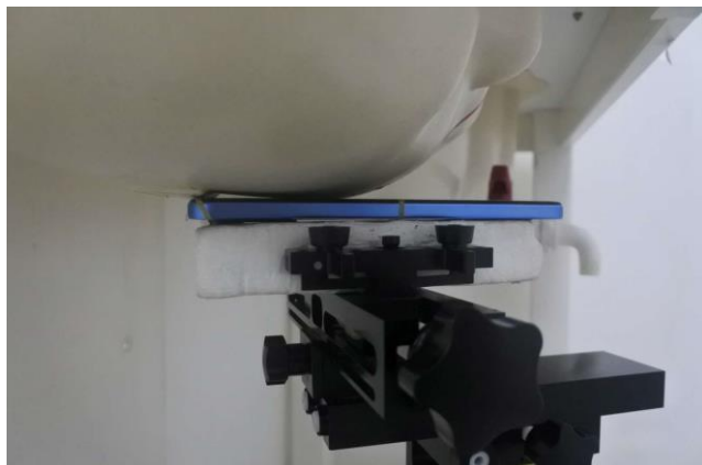
Right Cheek, Test Separation 0 mm
