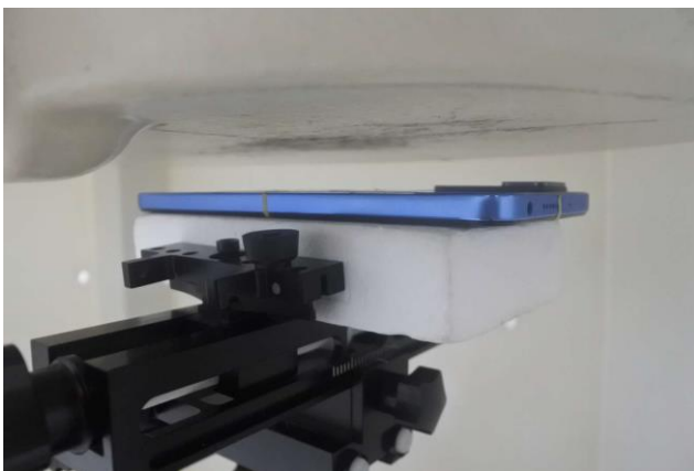
Back, Test Separation 20 mm(sensor off)
