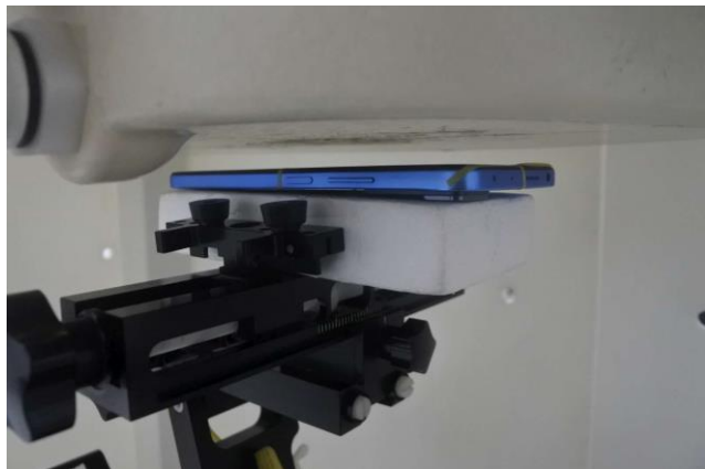
Front, Test Separation 10 mm
