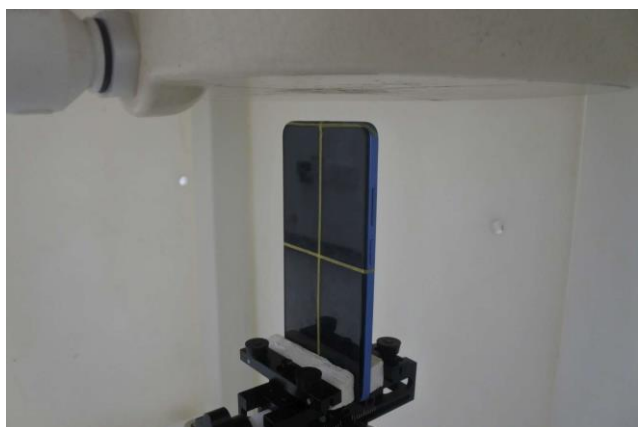
Top Side, Test Separation 15 mm(sensor off)
