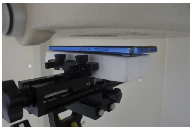
Front, Test Separation 15 mm(sensor off)
