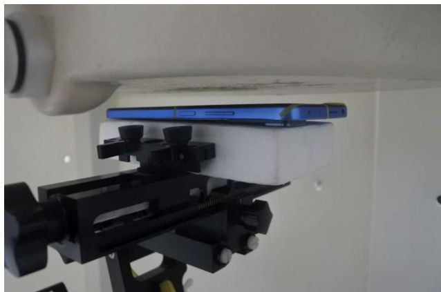
Front, Test Separation 10 mm
