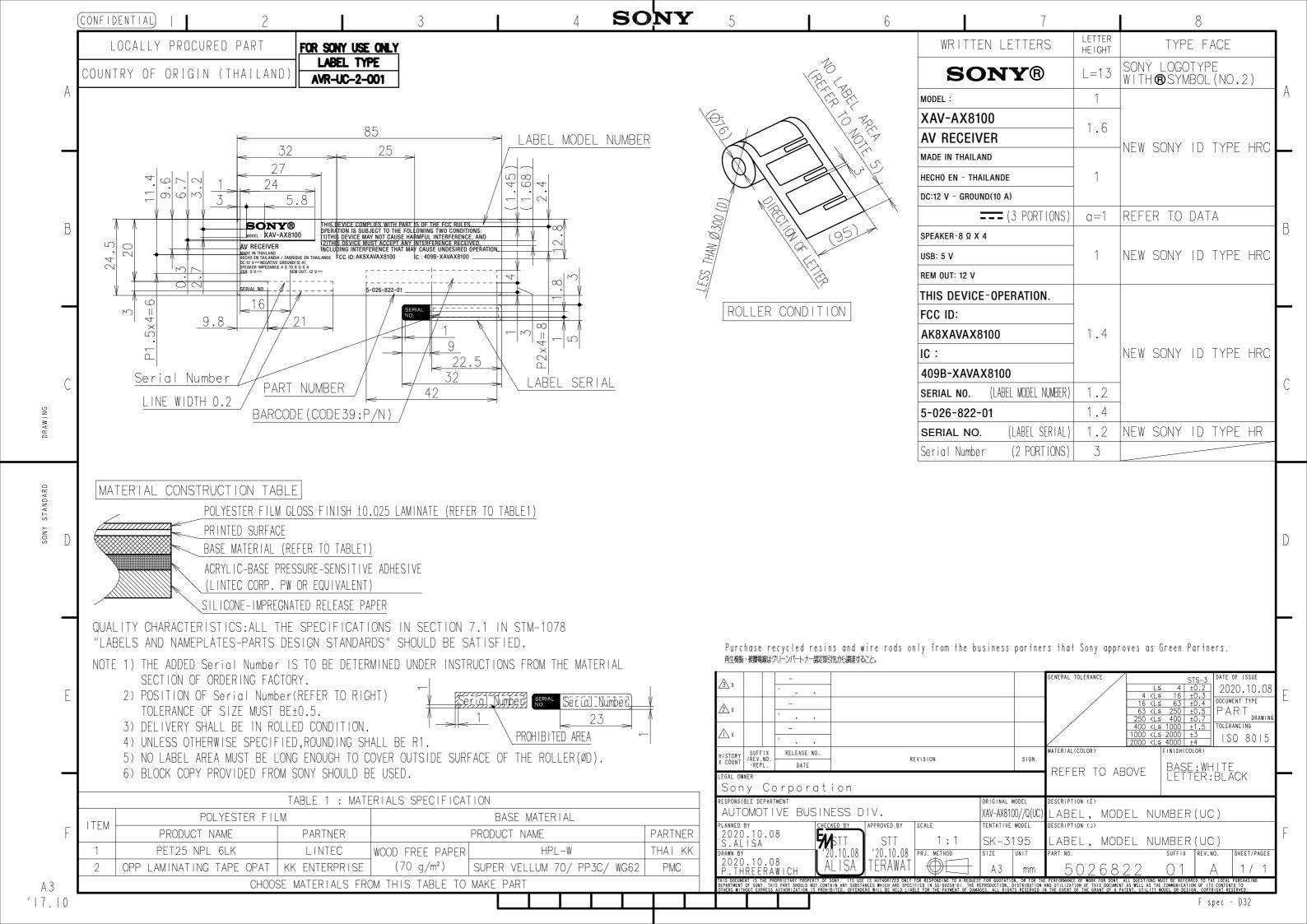
Type Approval mark label and serial number is to be printed are on the same plate label affixed to bottom of main unit
