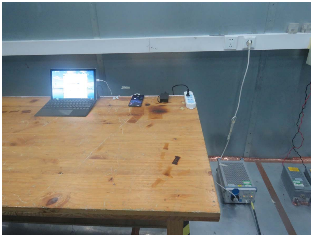
Picture 2: Conducted Emissions Test Setup
