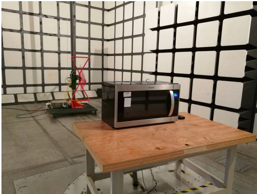
Radiated Emissions - Front View (30 MHz – 1 GHz)
