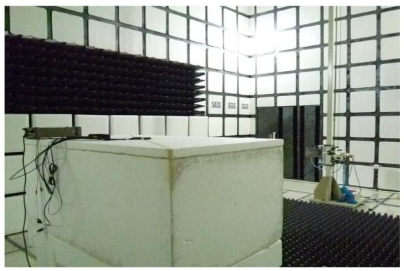
Radiated Emission Set up Photos (Front View)
