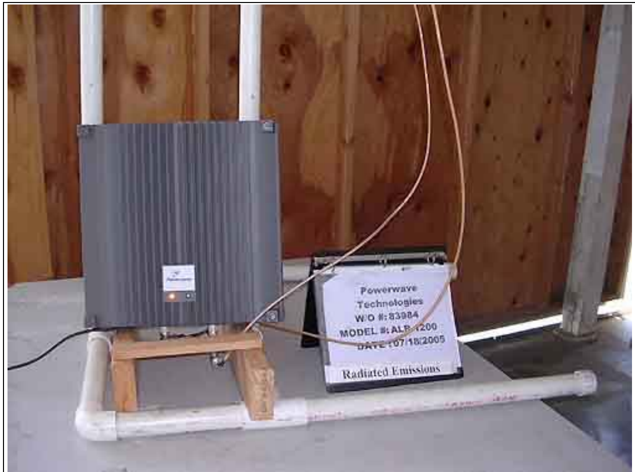
Radiated Emissions - Front View
