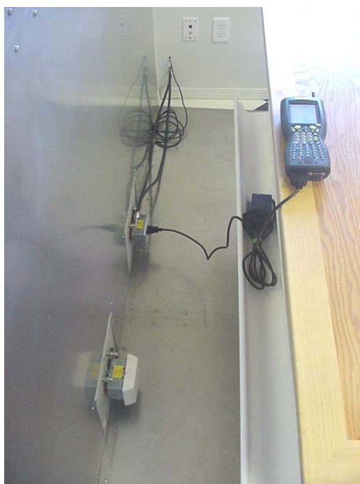
Photograph A.6-2 - AC Powerline Conducted Emissions Cable Placement
