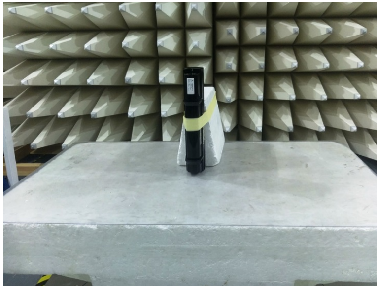
Photograph 8.1.3 Setup for radiated emission measurements, EUT cabling
