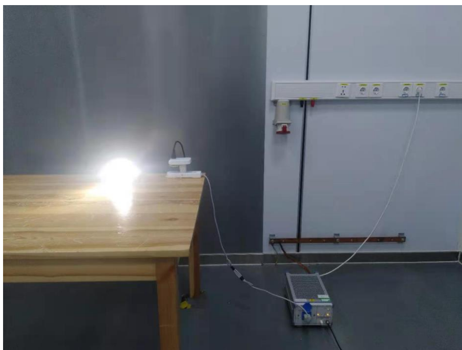
Fig. 4 Power line conducted emission setup photo
