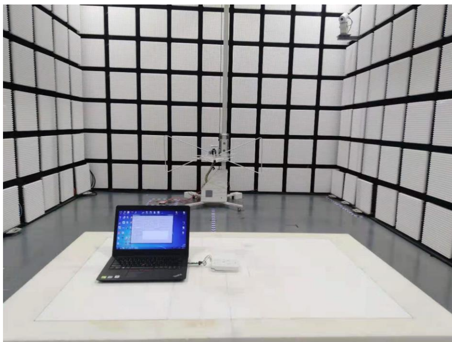
Fig. 2 Radiated emission setup photo(30MHz-1GHz)
