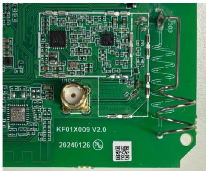
Figure 9 - GLOBYTNG3 radio module with internal antenna and without metallic shield
