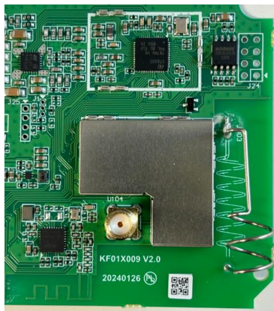
Figure 8 - GLOBYTNG3 radio module with internal antenna
