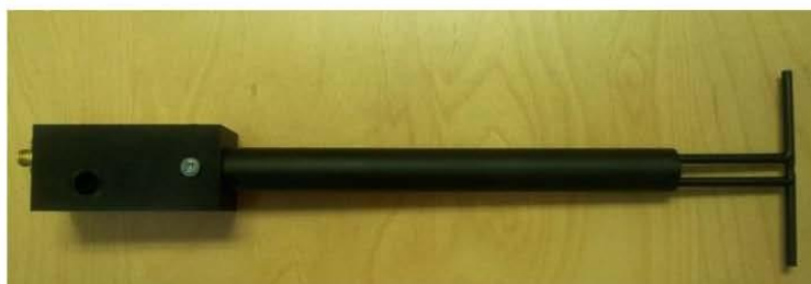
Figure 1 – MVG COMOSAR Validation Dipole
