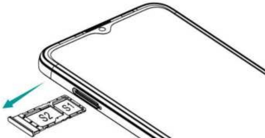
To eject SIM or MicroSD card, insert your SIM eject pin into the small hole next to the card tray.
