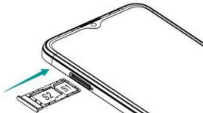
When inserting your card tray, make sure that the card is level and that the card is aligned correctly.
