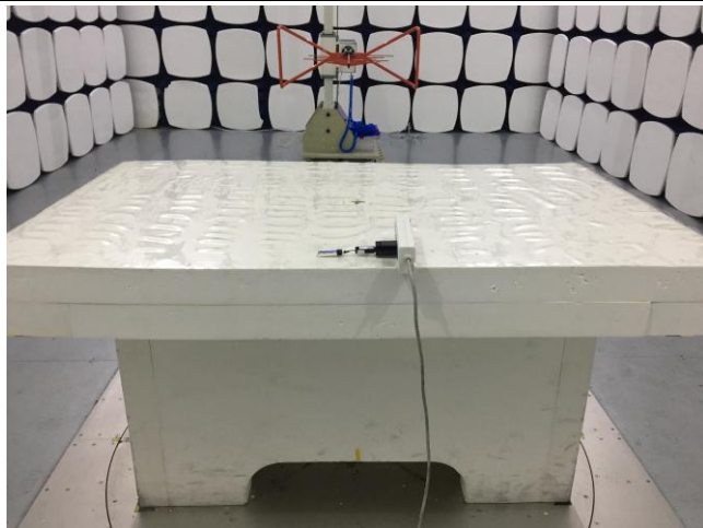
Radiated Emissions Test Setup Below 1GHz
