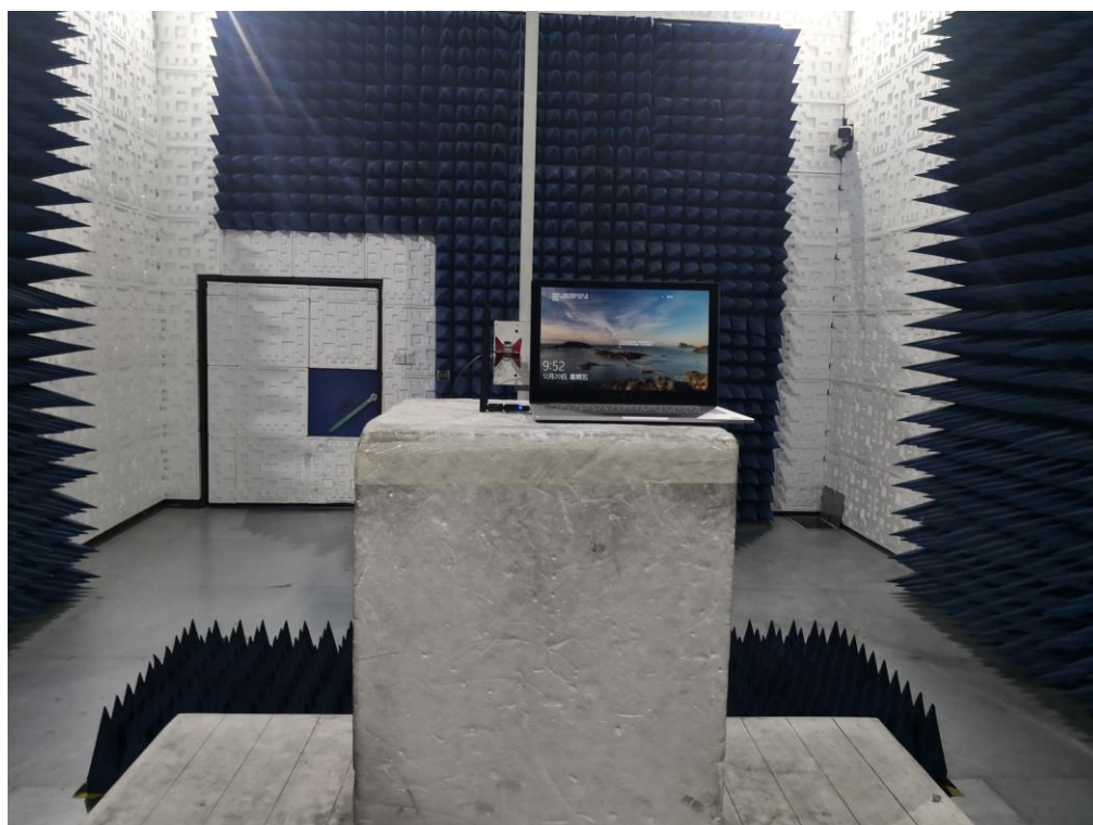
FCC RADIATED EMISSION TEST SETUP ABOVE 1GHZ
