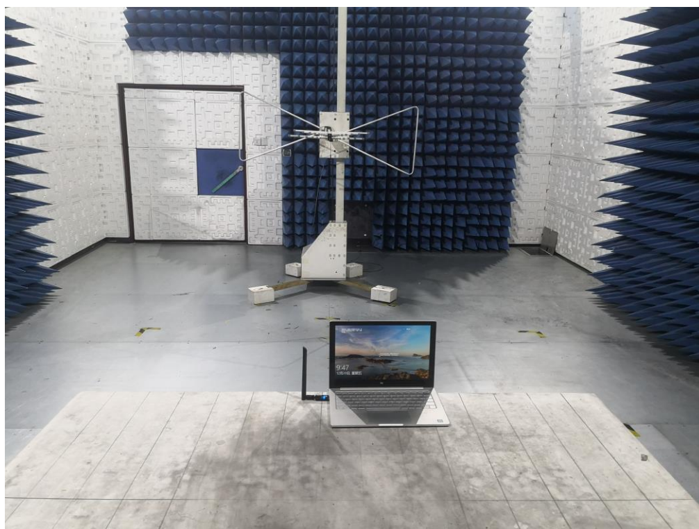
FCC RADIATED EMISSION TEST SETUP ABOVE 1GHZ
