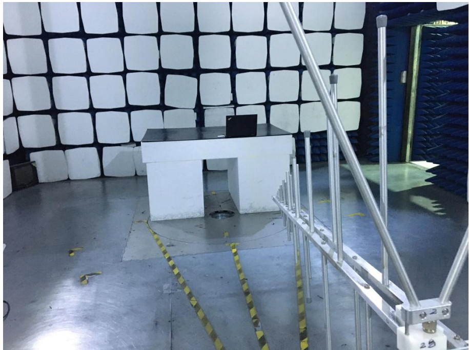
Radiation Emission Test Setup (30MHz to 1GHz)
