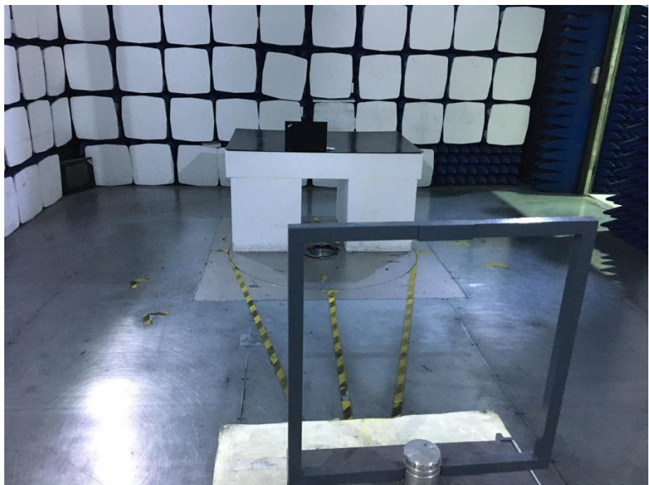
Radiation Emission Test Setup (Below 30MHz)
