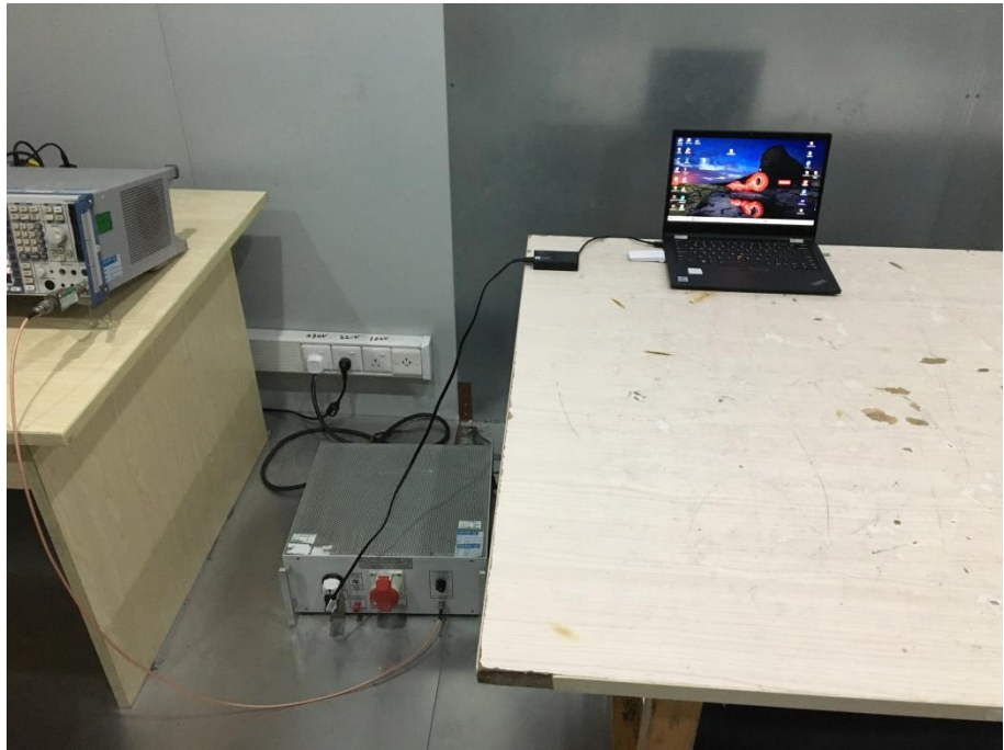
Conducted Emission Test Setup
