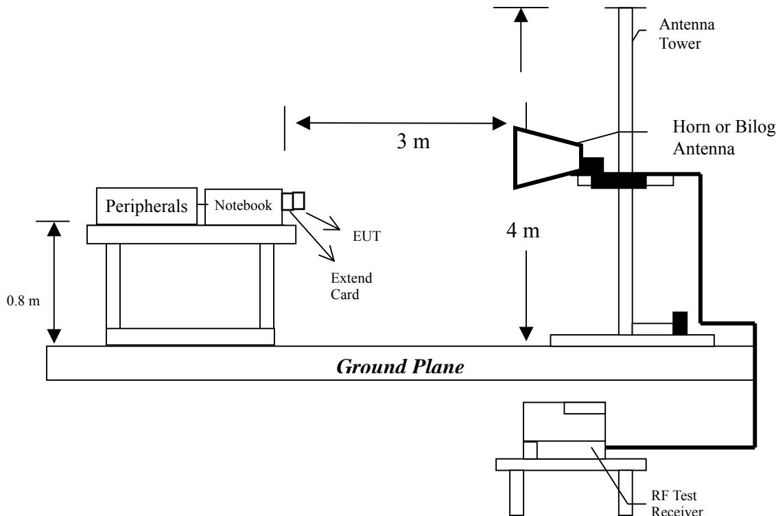
Radiated emission measurements were performed from 30MHz to 25GHz. Spectrum Analyzer Resolution Bandwidth is 100kHz or greater for frequencies 30MHz to 1GHz, 1MHz – for frequencies above 1GHz.
