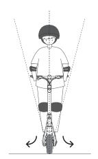
6. To stop, release the rotary handle to slow down and squeeze the brake lever. Unfold the kickstand and let the vehicle lean slightly so that the kickstand meets the ground, and then the vehicle can be placed stably.
