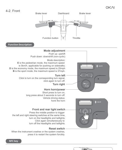
In the offff state, the NFC key card is close to the screen to turn on and unlock;
