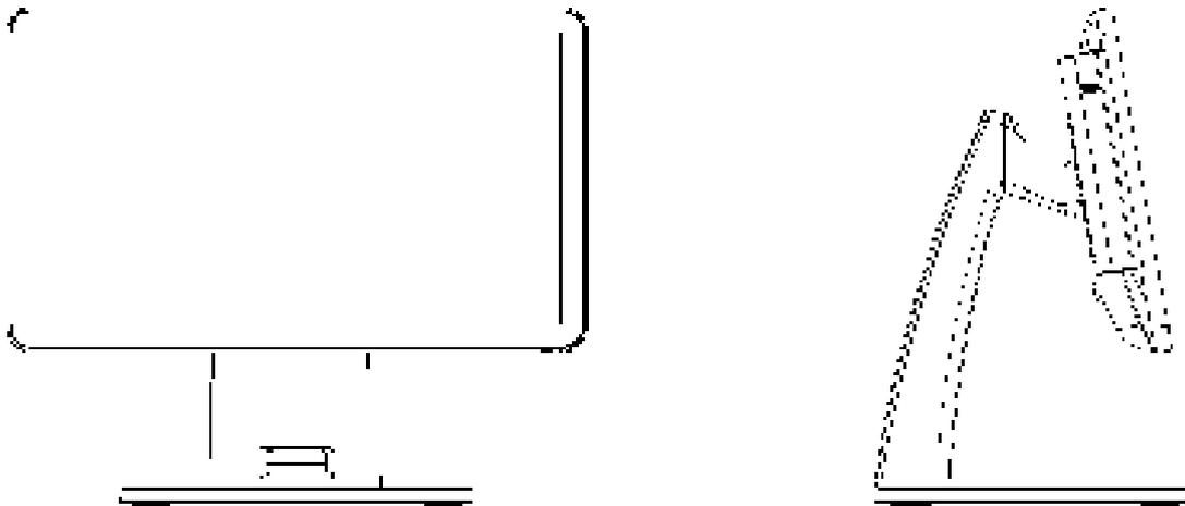
Single screen, length×width×height: 380mm\*198mm\*327mm; main screen flip angle 0-45°
