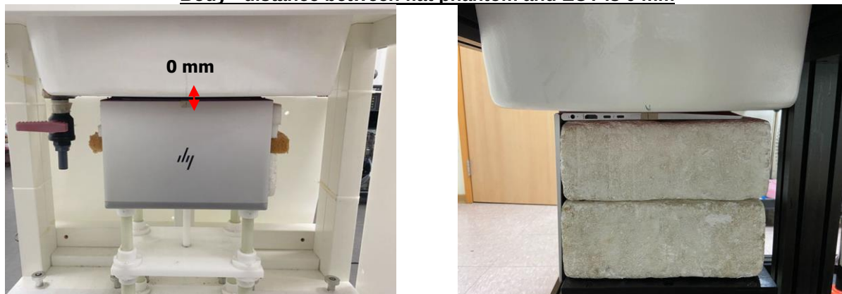
Fig.3 EUT Bottom side to flat phantom
