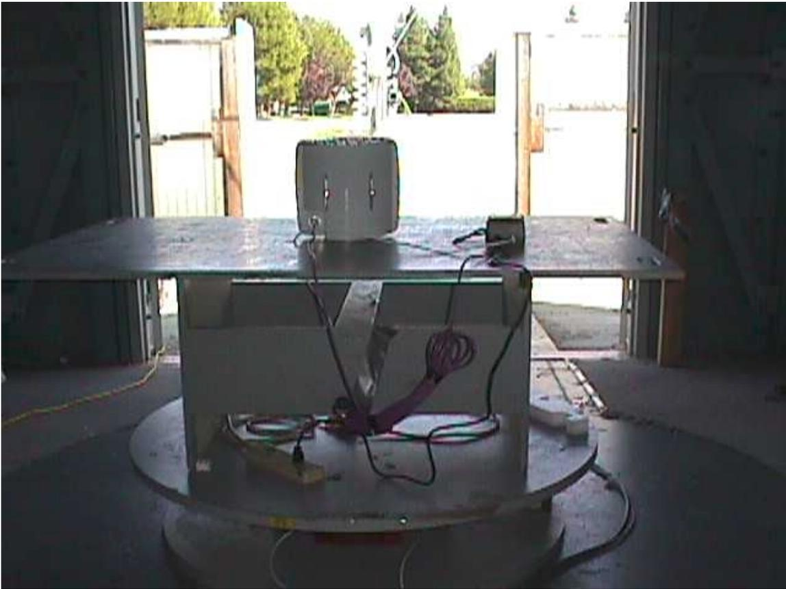
AC Line conducted emission test
