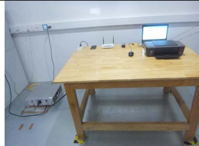
Conducted Emissions Test Setup – Front View
