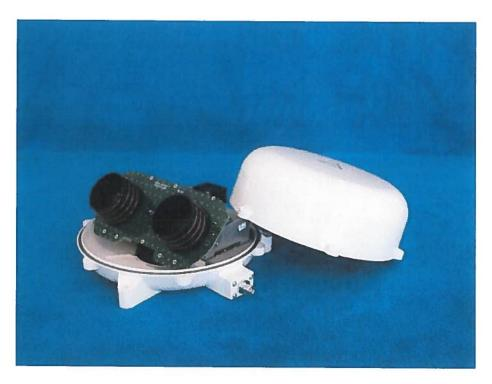
For Class 16 Operation the active antenna is developed by Honeywell, patent pending. It is of a crooked wire design, omnidirectional, working down to 5° elevation.
