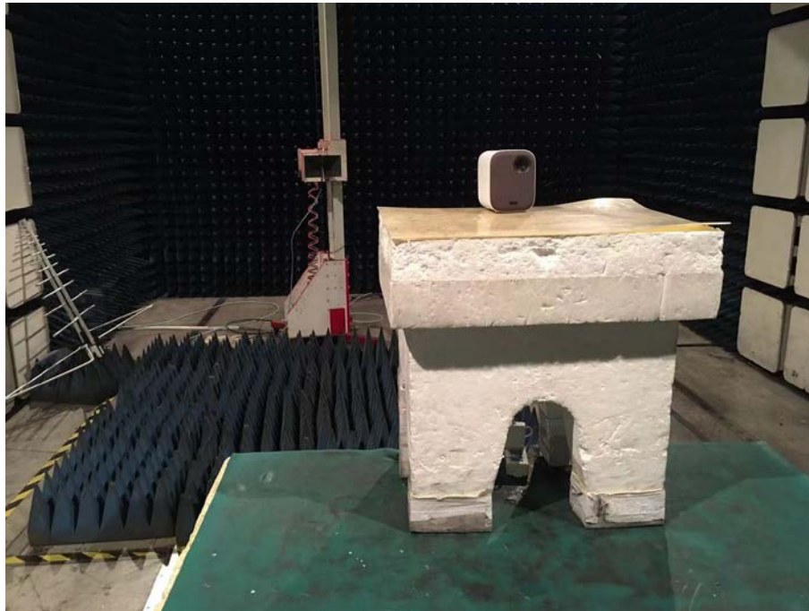
Spurious Emission Test Setup (Above 1GHz)
