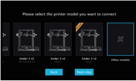
2.2 The printer needs to flash the self-compiled firmware first, then save the corresponding configuration file Printer.cfg into the USB drive, insert the Creality Sonic Pad, and click Next step.
