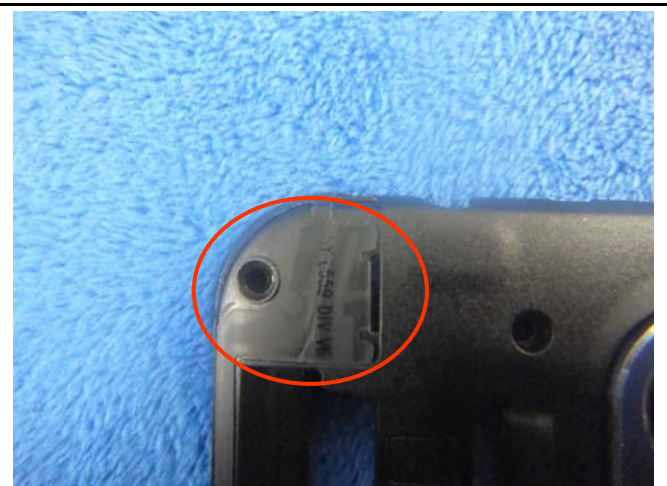
LTE - Antenna View
