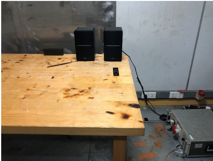
Photograph 3: Set-up for Conducted Emission on AC Mains
