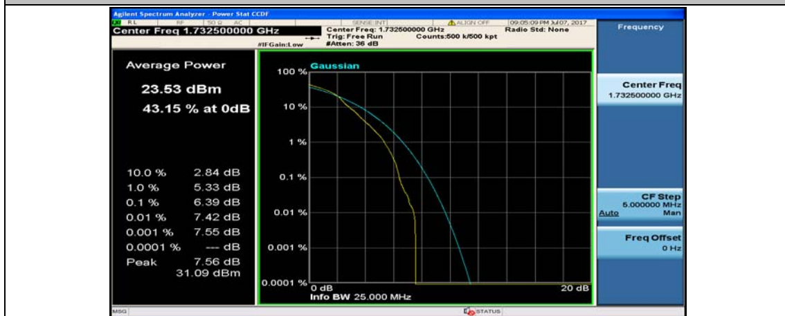
(Channel Bandwidth:20 MHz)_MCH_16QAM_1RB#49
