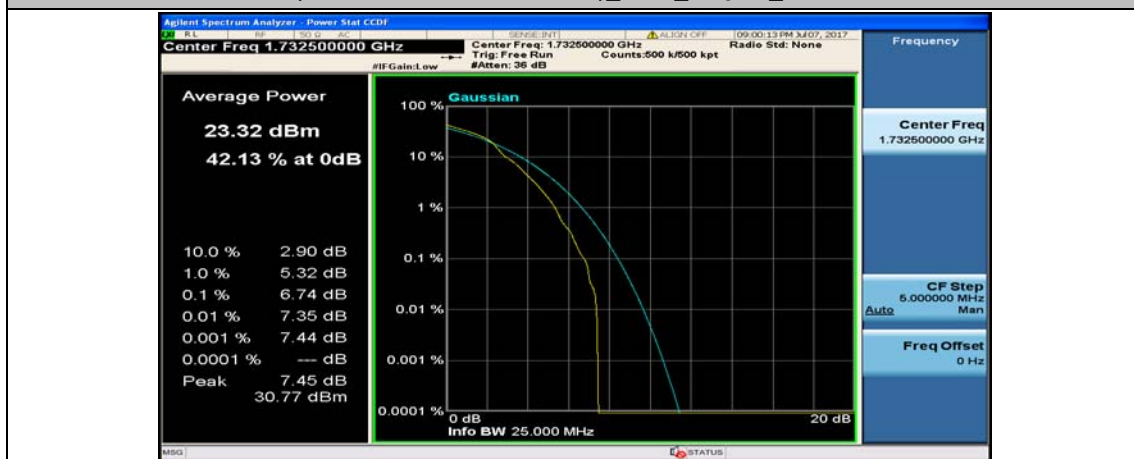
(Channel Bandwidth:15 MHz)_MCH_16QAM_1RB#37
