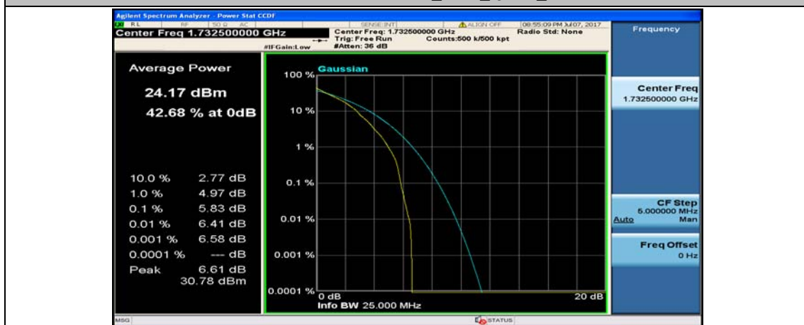
Channel Bandwidth: 10 MHz_MCH_QPSK_1RB#24
