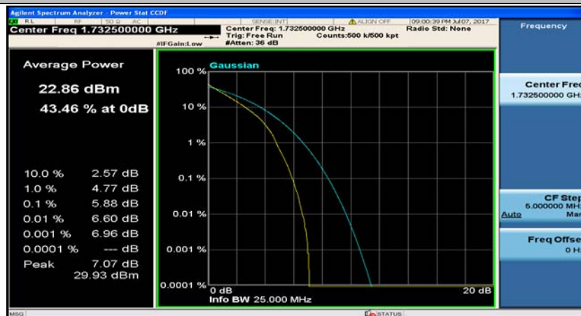
(Channel Bandwidth:15 MHz)_MCH_QPSK_37RB#38
