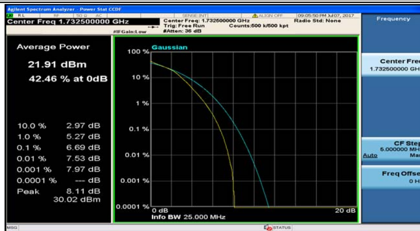
(Channel Bandwidth:20 MHz)_MCH_16QAM_50RB#25
