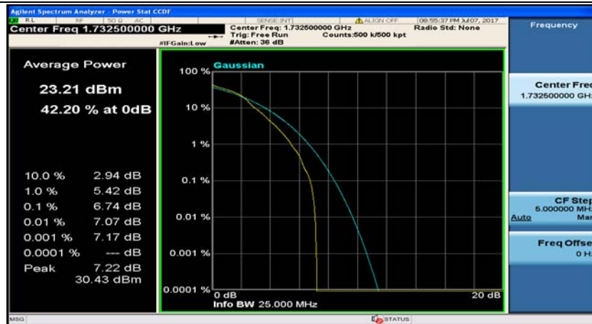
Channel Bandwidth: 10 MHz_MCH_16QAM_25RB#0
