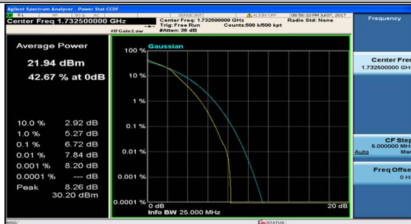
Channel Bandwidth: 10 MHz_MCH_16QAM_25RB#25
