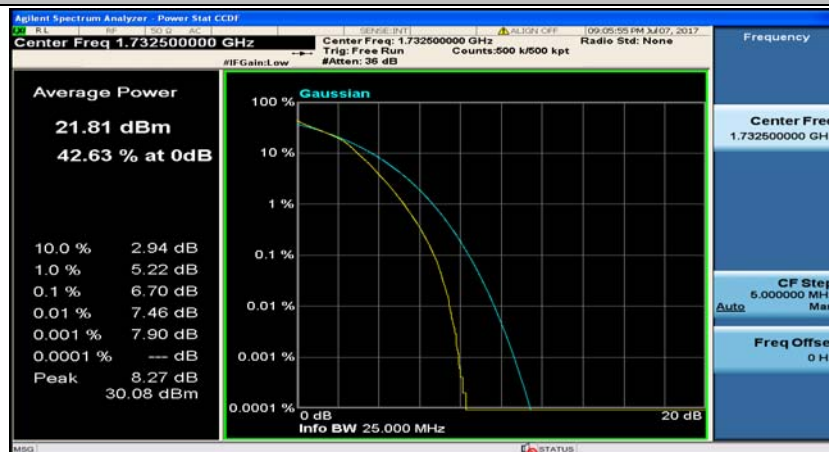
(Channel Bandwidth:20 MHz)_MCH_16QAM_50RB#50
