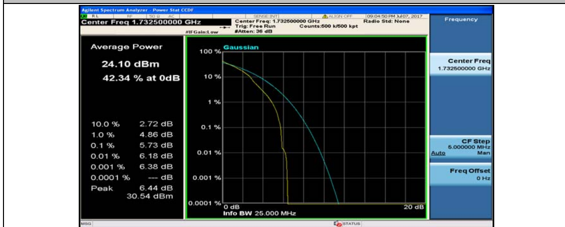
(Channel Bandwidth:20 MHz)_MCH_QPSK_1RB#49
