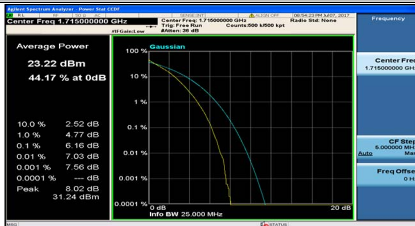
Channel Bandwidth: 10 MHz_LCH_QPSK_50RB#0
