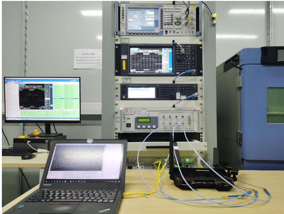
Photograph 3: Set-up photo for RF Conducted Singal test
