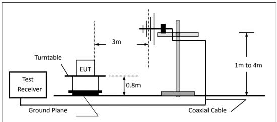
(c) For radiated emissions above 1000MHz
