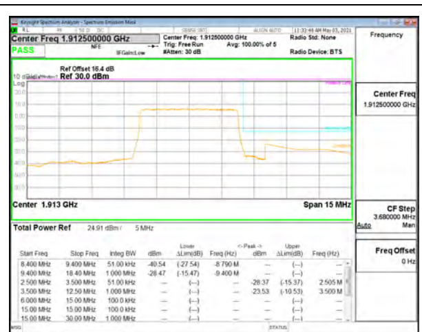
LTE B25 5MHz QPSK High Channel RB25-0
