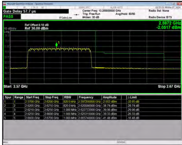
n38 SCS=30kHz DFT_64QAM BW=40MHz HighChannel=520000 RB=100@0
