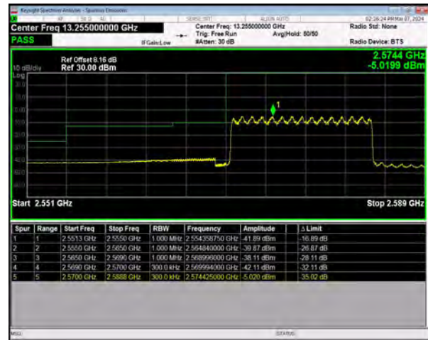
n38 SCS=30kHz DFT_256QAM BW=15MHz LowChannel=515500 RB=36@0
