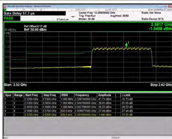
n38 SCS=30kHz DFT_16QAM BW=40MHz LowChannel=518000 RB=100@0
