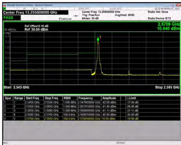
n38 SCS=30kHz DFT_BPSK BW=20MHz LowChannel=516000 RB=1@0
