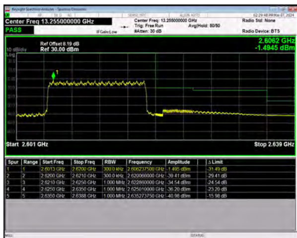
n38 SCS=30kHz DFT_16QAM BW=15MHz HighChannel=522500 RB=36@0
