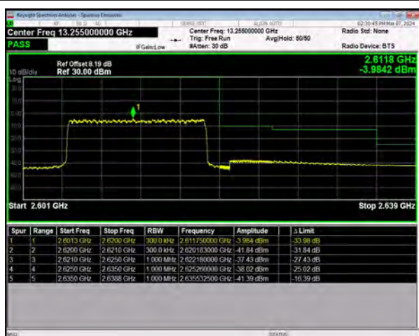
n38 SCS=30kHz DFT_64QAM BW=15MHz HighChannel=522500 RB=36@0
