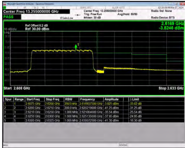
n38 SCS=30kHz DFT_64QAM BW=10MHz HighChannel=523000 RB=24@0
