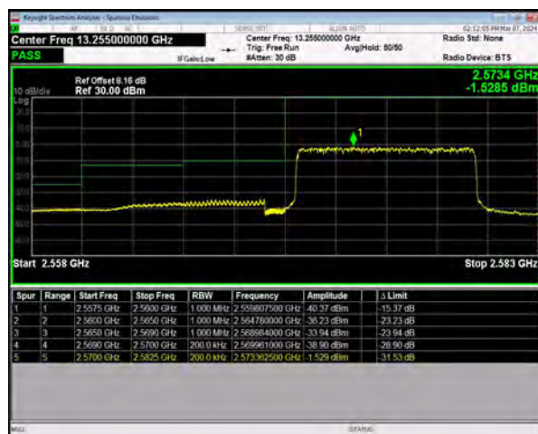
n38 SCS=30kHz DFT_BPSK BW=10MHz LowChannel=515000 RB=24@0
