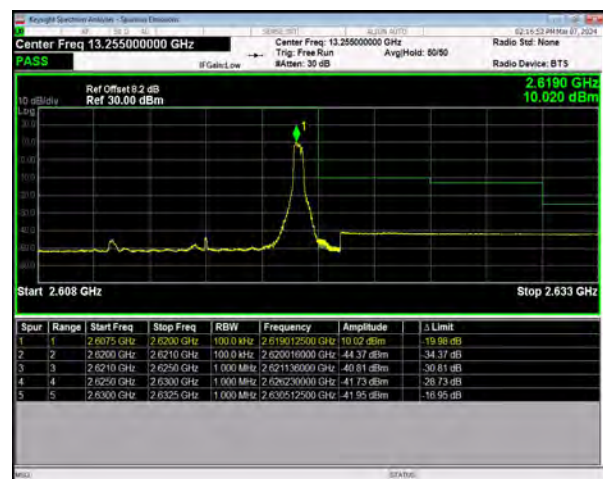
n38 SCS=30kHz DFT_BPSK BW=10MHz HighChannel=523000 RB=1@23
