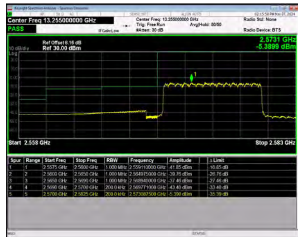
n38 SCS=30kHz DFT_256QAM BW=10MHz LowChannel=515000 RB=24@0
