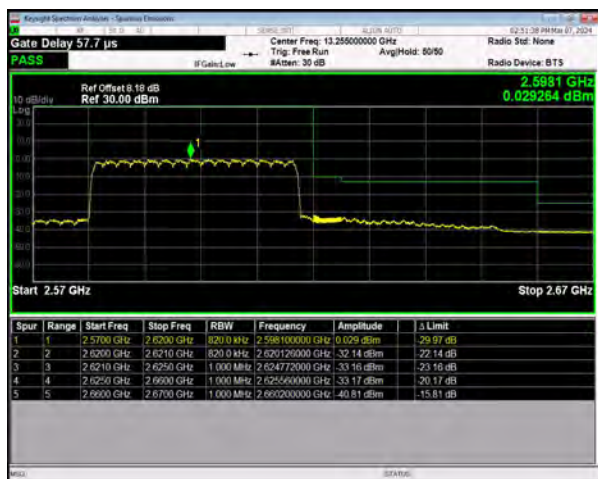
n38 SCS=30kHz DFT_QPSK BW=40MHz HighChannel=520000 RB=100@0
