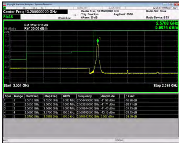
n38 SCS=30kHz DFT_256QAM BW=15MHz LowChannel=515500 RB=1@0
