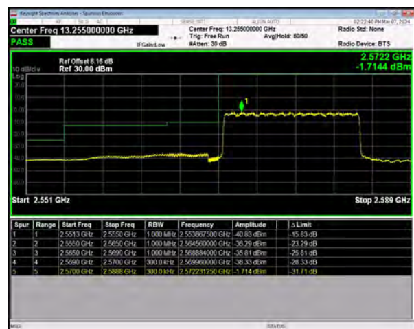
n38 SCS=30kHz DFT_BPSK BW=15MHz LowChannel=515500 RB=36@0
