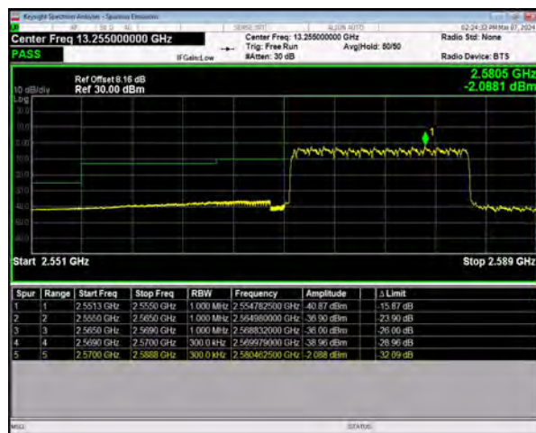
n38 SCS=30kHz DFT_16QAM BW=15MHz LowChannel=515500 RB=36@0
