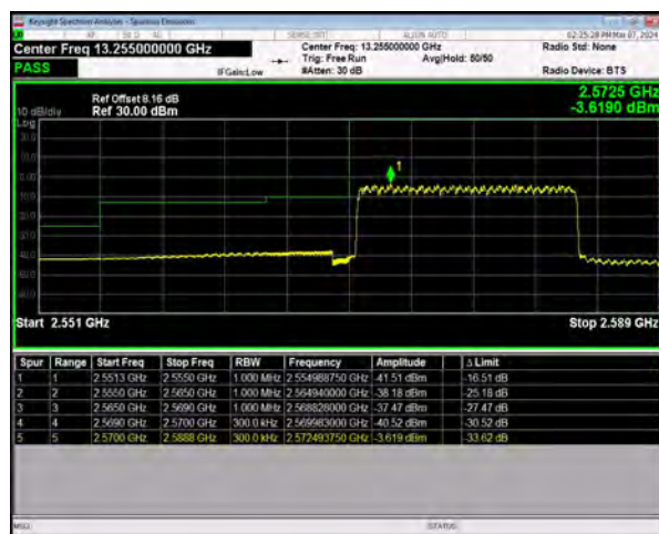
n38 SCS=30kHz DFT_64QAM BW=15MHz LowChannel=515500 RB=36@0
