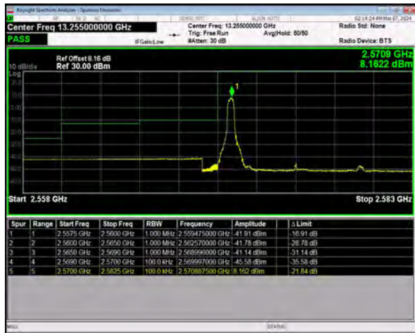
n38 SCS=30kHz DFT_64QAM BW=10MHz LowChannel=515000 RB=1@0
