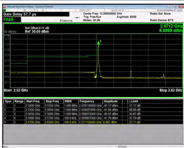
n38 SCS=30kHz DFT_16QAM BW=40MHz LowChannel=518000 RB=1@0
