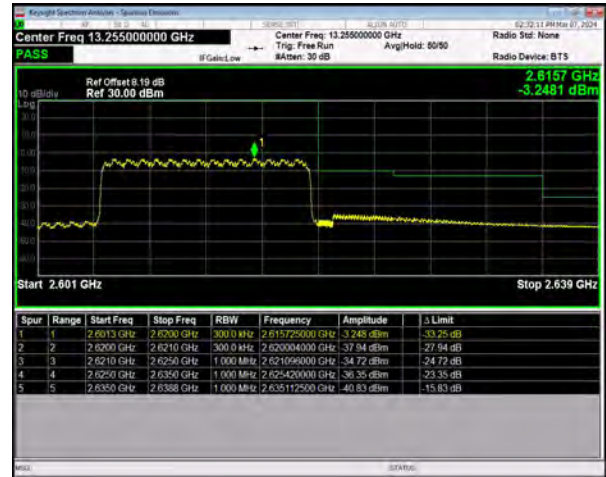
n38 SCS=30kHz CP_QPSK BW=15MHz HighChannel=522500 RB=38@0
