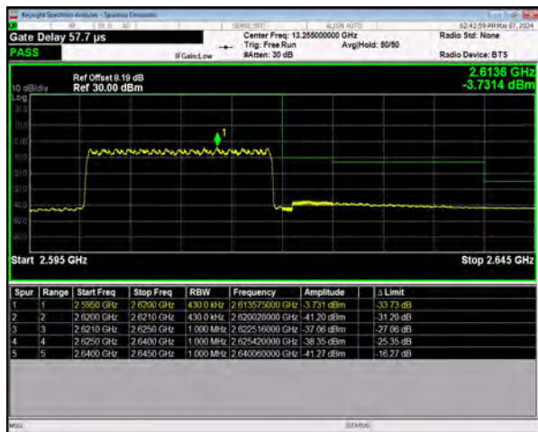
n38 SCS=30kHz DFT_64QAM BW=20MHz HighChannel=522000 RB=50@0
