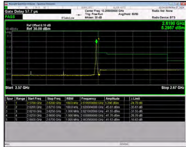
n38 SCS=30kHz DFT_256QAM BW=40MHz HighChannel=520000 RB=1@105
