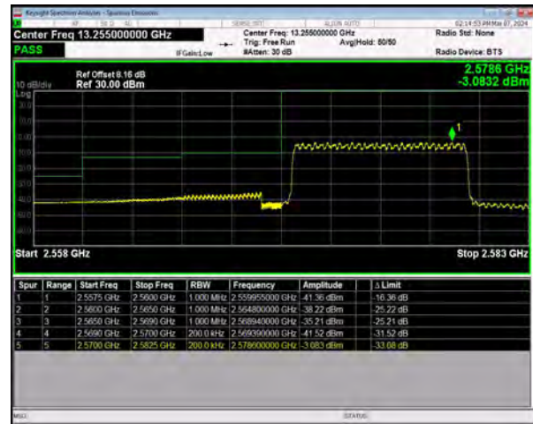
n38 SCS=30kHz DFT_64QAM BW=10MHz LowChannel=515000 RB=24@0
