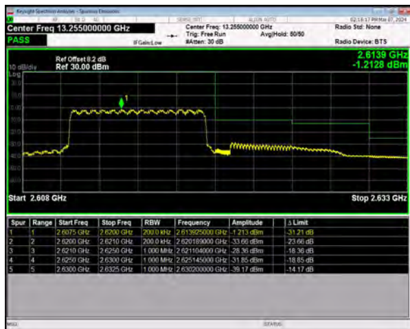
n38 SCS=30kHz DFT_QPSK BW=10MHz HighChannel=523000 RB=24@0
