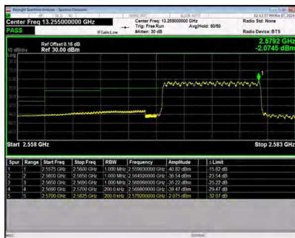
n38 SCS=30kHz DFT_16QAM BW=10MHz LowChannel=515000 RB=24@0
