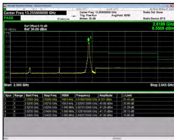
n38 SCS=30kHz DFT_BPSK BW=20MHz HighChannel=522000 RB=1@50
