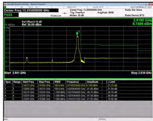
n38 SCS=30kHz DFT_BPSK BW=15MHz HighChannel=522500 RB=1@37
