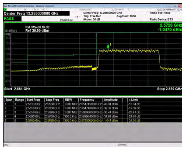
n38 SCS=30kHz DFT_QPSK BW=15MHz LowChannel=515500 RB=36@0
