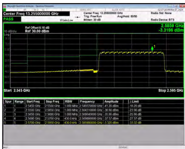
n38 SCS=30kHz CP_QPSK BW=20MHz LowChannel=516000 RB=51@0
