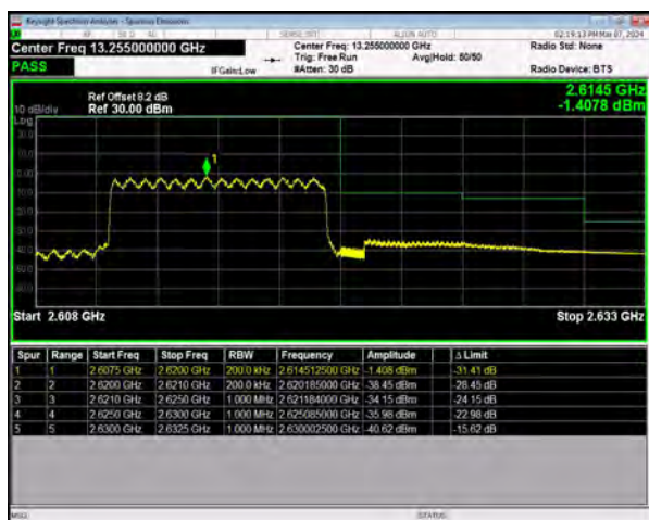
n38 SCS=30kHz DFT_16QAM BW=10MHz HighChannel=523000 RB=24@0
