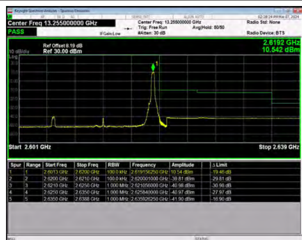
n38 SCS=30kHz DFT_QPSK BW=15MHz HighChannel=522500 RB=1@37
