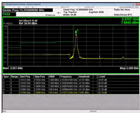
n38 SCS=30kHz DFT_16QAM BW=15MHz LowChannel=515500 RB=1@0
