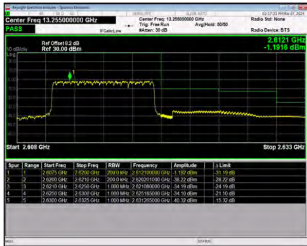
n38 SCS=30kHz DFT_BPSK BW=10MHz HighChannel=523000 RB=24@0
