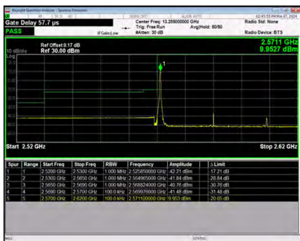
n38 SCS=30kHz DFT_QPSK BW=40MHz LowChannel=518000 RB=1@0
