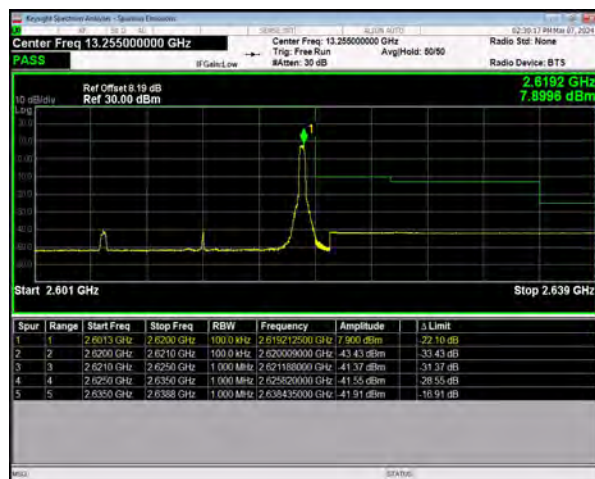
n38 SCS=30kHz DFT_64QAM BW=15MHz HighChannel=522500 RB=1@37
