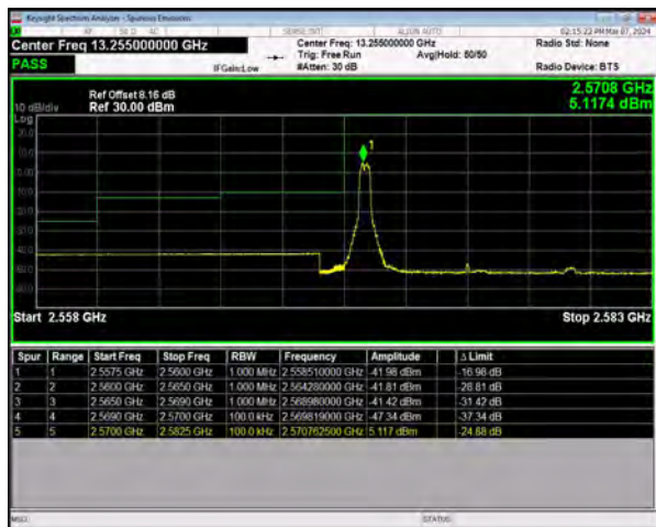
n38 SCS=30kHz DFT_256QAM BW=10MHz LowChannel=515000 RB=1@0
