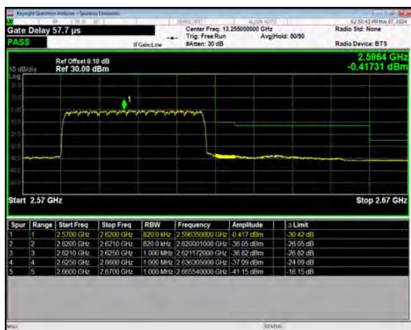
n38 SCS=30kHz DFT_BPSK BW=40MHz HighChannel=520000 RB=100@0
