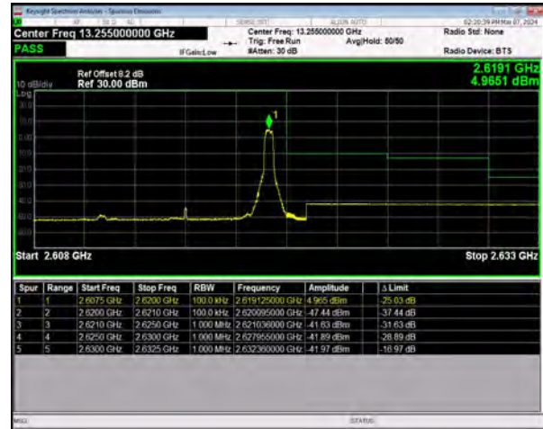
n38 SCS=30kHz DFT_256QAM BW=10MHz HighChannel=523000 RB=1@23
