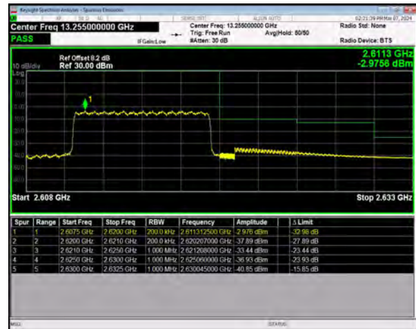
n38 SCS=30kHz CP_QPSK BW=10MHz HighChannel=523000 RB=24@0
