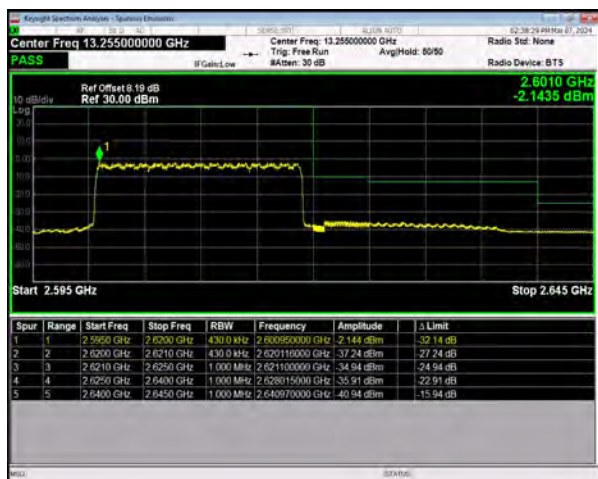
n38 SCS=30kHz DFT_BPSK BW=20MHz HighChannel=522000 RB=50@0
