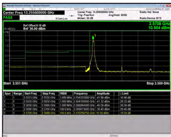
n38 SCS=30kHz DFT_BPSK BW=15MHz LowChannel=515500 RB=1@0
