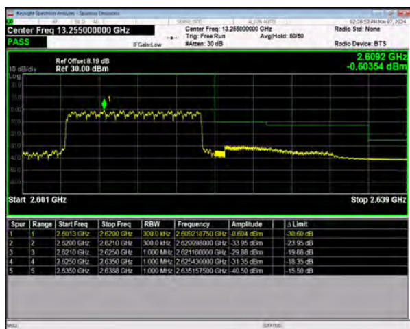
n38 SCS=30kHz DFT_QPSK BW=15MHz HighChannel=522500 RB=36@0
