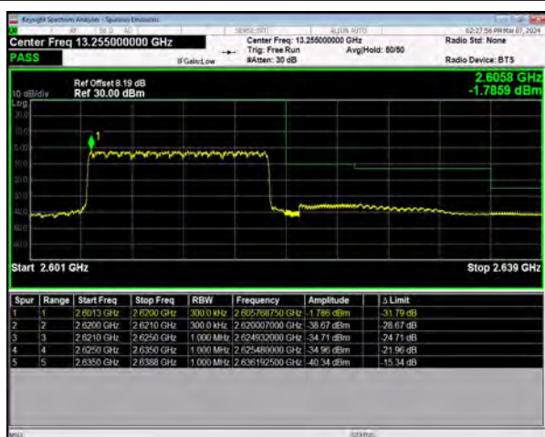
n38 SCS=30kHz DFT_BPSK BW=15MHz HighChannel=522500 RB=36@0
