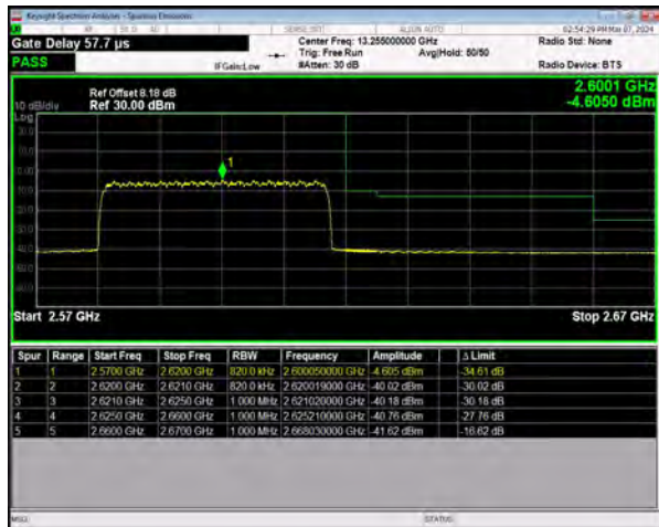
n38 SCS=30kHz DFT_256QAM BW=40MHz HighChannel=520000 RB=100@0
