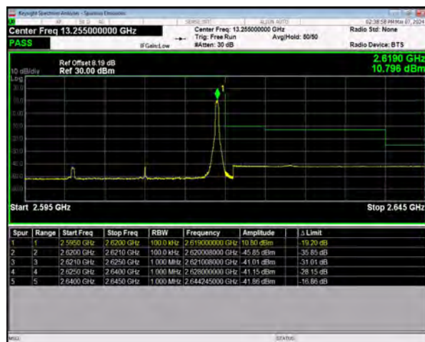
n38 SCS=30kHz DFT_QPSK BW=20MHz HighChannel=522000 RB=1@50
