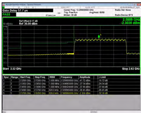
n38 SCS=30kHz CP_QPSK BW=40MHz LowChannel=518000
