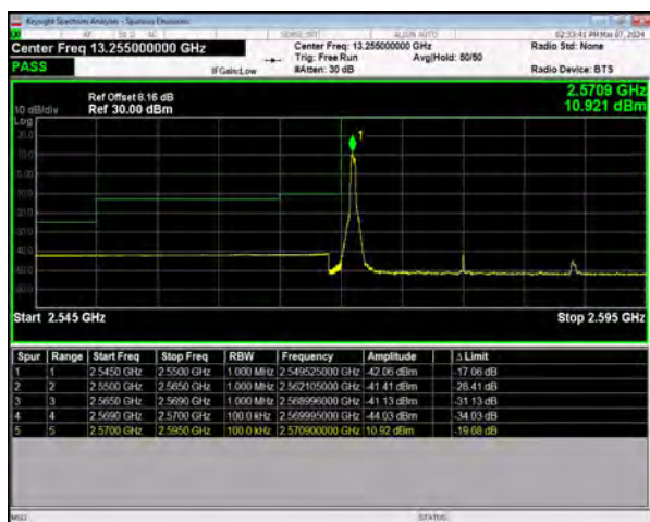
n38 SCS=30kHz DFT_QPSK BW=20MHz LowChannel=516000 RB=1@0
