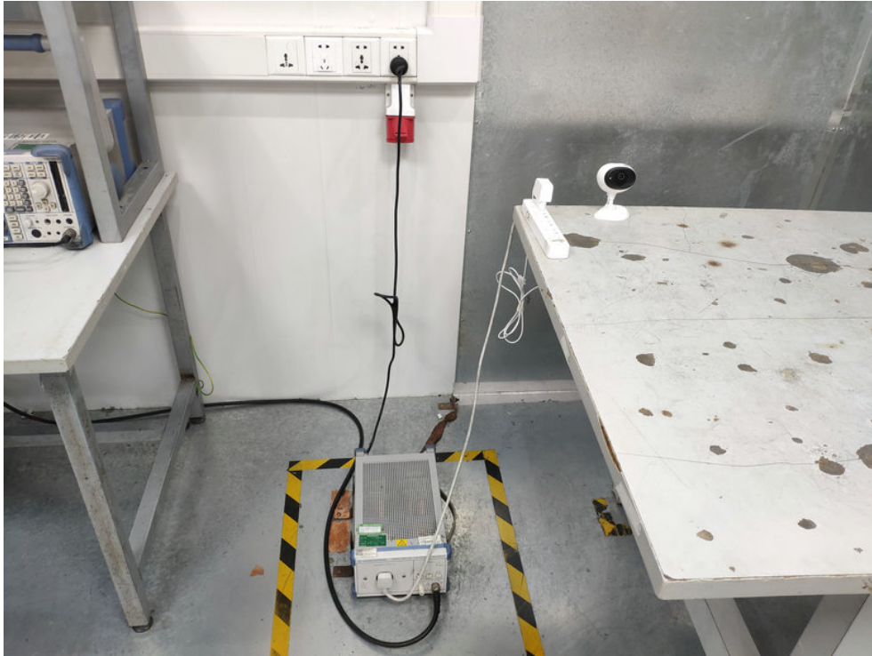
Photo of Conducted Emission Measurement
