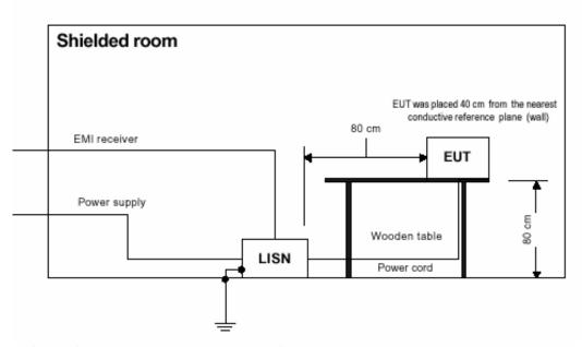
Setup for mains terminal radio interference voltage test, table-top equipment
