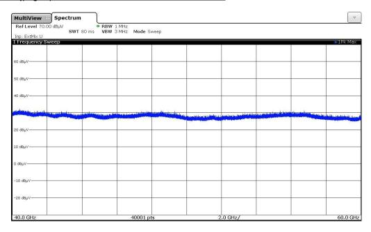
No emission above noise floor of the measuring system (77.1 dB $\mu$ V/m measured with peak detector with 0.1 m measuring distance) found in this frequency range.
