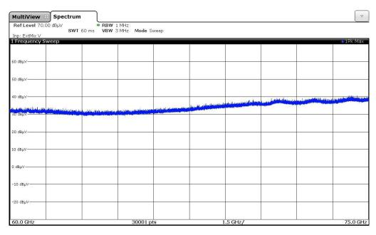
No emission above noise floor of the measuring system (69 dB $\mu$ V/m measured with peak detector with 0.1 m measuring distance) found in this frequency range.
