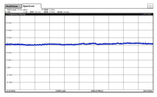
No emission above noise floor of the measuring system (45 dB $\mu$ V/m measured with peak detector with 3 m measuring distance) found in this frequency range.
