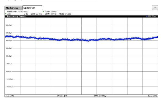
No emission above noise floor of the measuring system (50.2 dB $\mu$ V/m) measured with peak detector with 3 m measuring distance) found in this frequency range.
