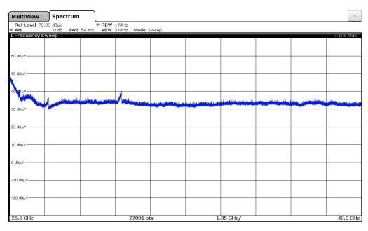
No emission above noise floor of the measuring system (56 dB $\mu$ V/m measured with peak detector with 1 m measuring distance) found in this frequency range.
