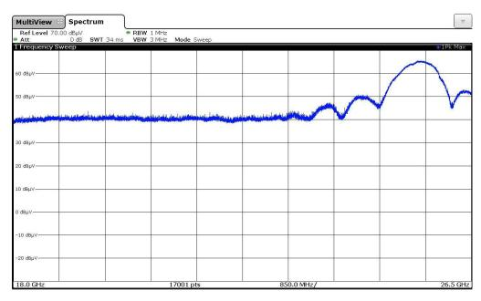
No emission above noise floor of the measuring system (48 dBµV/m measured with peak detector with 3 m measuring distance) except the wanted signal of the LPR device found in this frequency range.
