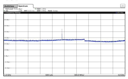
No emission above noise floor of the measuring system (61 dB $\mu$ V/m measured with peak detector with 3 m measuring distance) except the wanted signal of the Bluetooth Low Energy device found in this frequency range.
