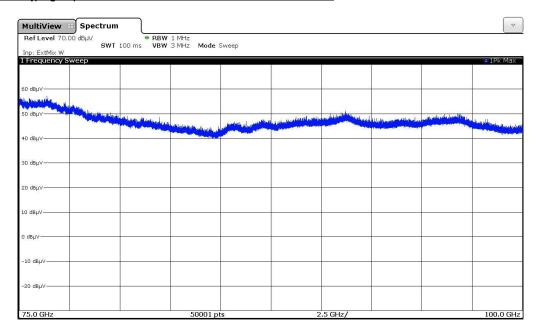
No emission above noise floor of the measuring system (105 dB $\mu$ V/m measured with peak detector with 0.03 m measuring distance) found in this frequency range.
