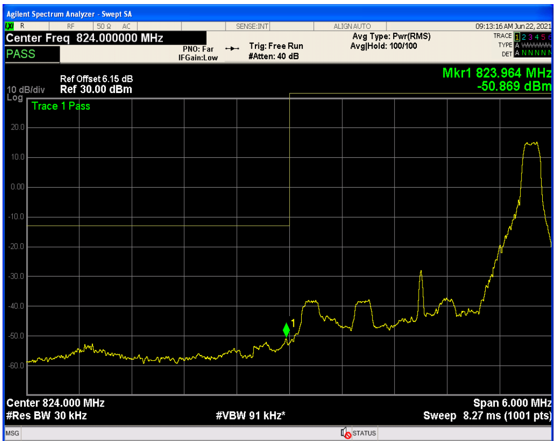
Band5 QPSK BW=3MHz Channel=20635 RB Size=1 Position=#0
