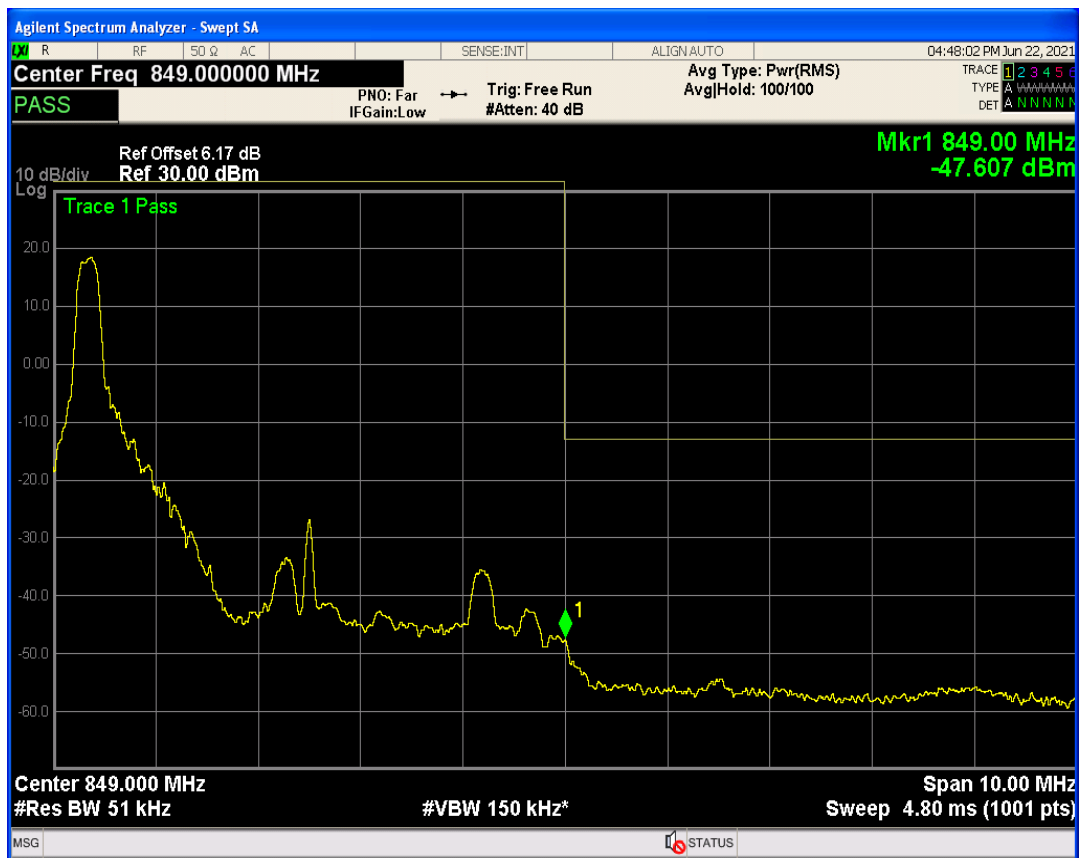
Band26b QPSK BW=5MHz Channel=27015 RB Size=1 Position=#Max
