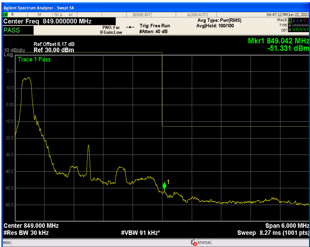
Band26b QPSK BW=3MHz Channel=27025 RB Size=15 Position=#0
