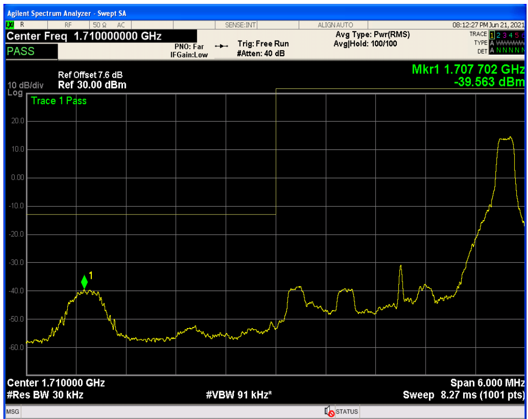
Band4 QPSK BW=3MHz Channel=20385 RB Size=1 Position=#0
