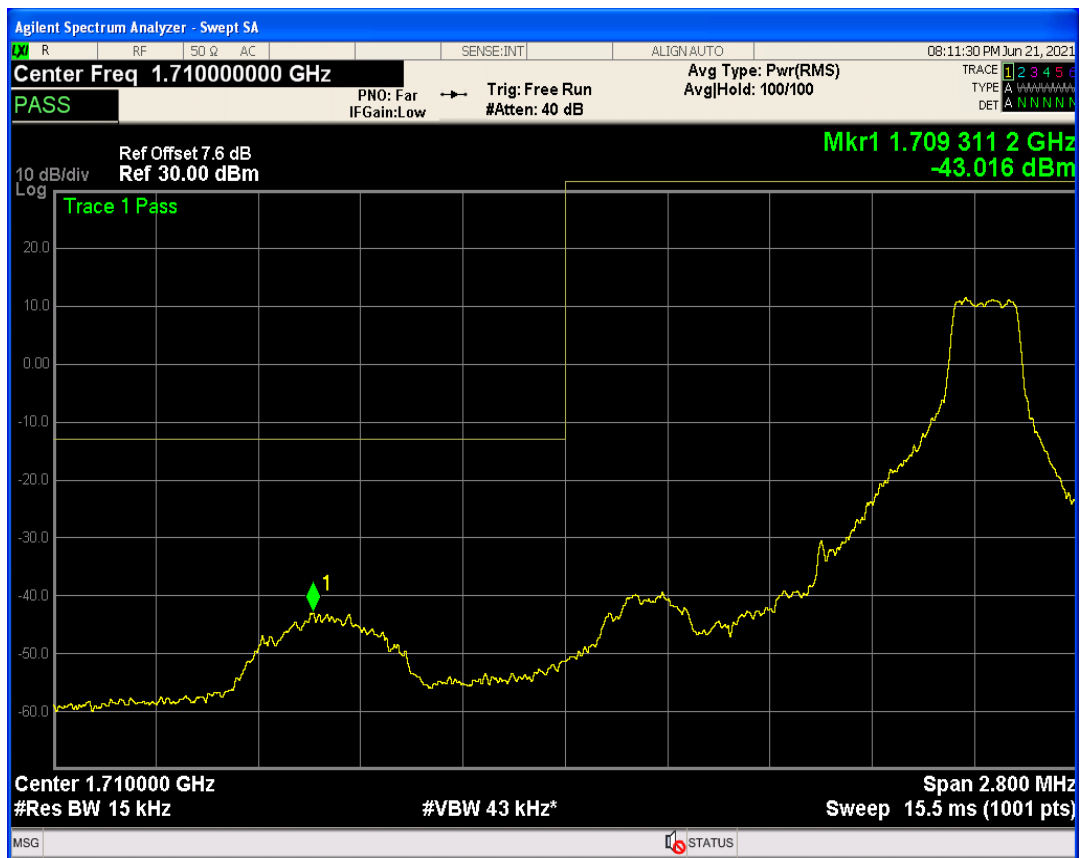
Band4 QAM16 BW=1.4MHz Channel=19957 RB Size=6 Position=#0
