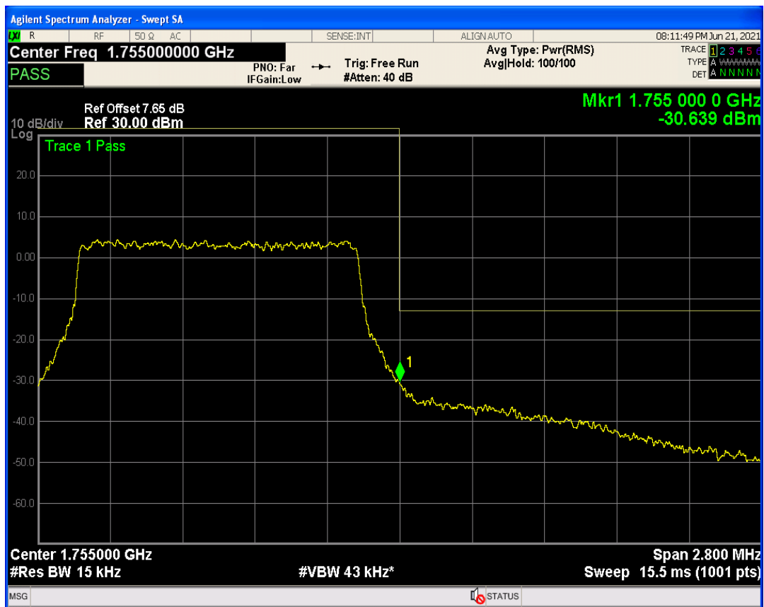
Band4 QAM16 BW=1.4MHz Channel=20393 RB Size=1 Position=#0
