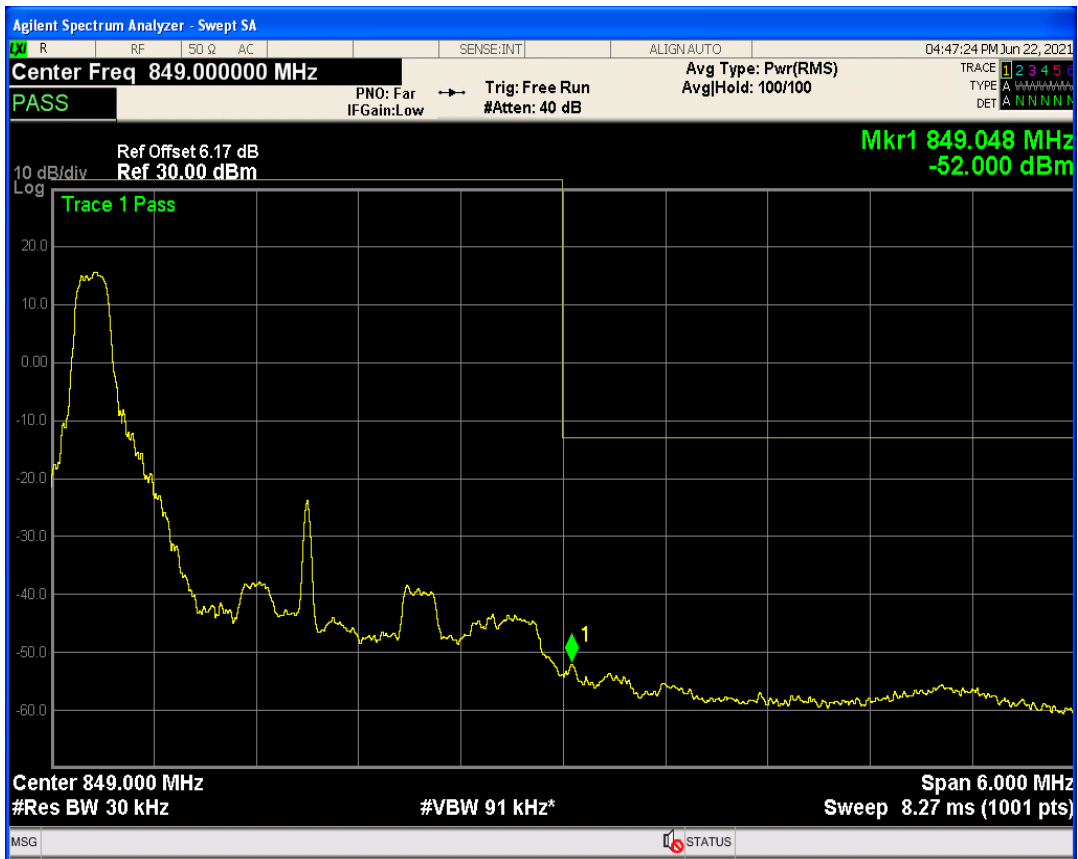
Band26b QAM16 BW=3MHz Channel=27025 RB Size=15 Position=#0
