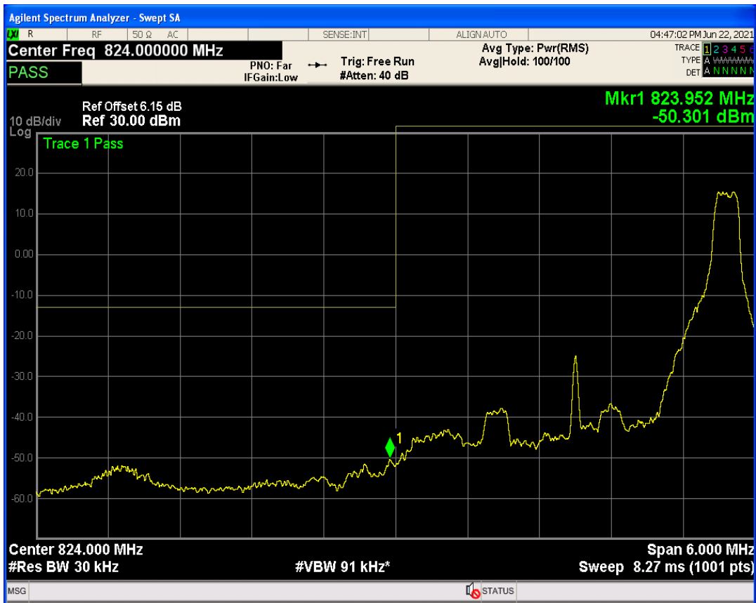
Band26b QPSK BW=3MHz Channel=27025 RB Size=1 Position=#0
