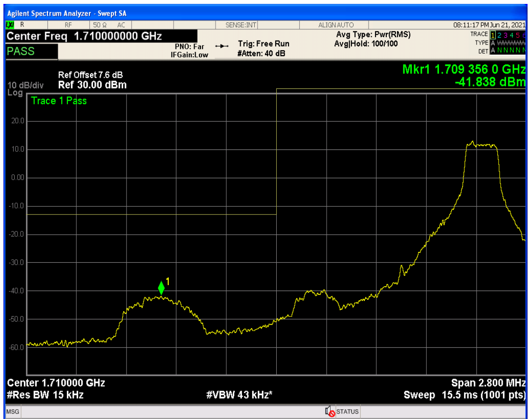
Band4 QPSK BW=1.4MHz Channel=19957 RB Size=1 Position=#0
