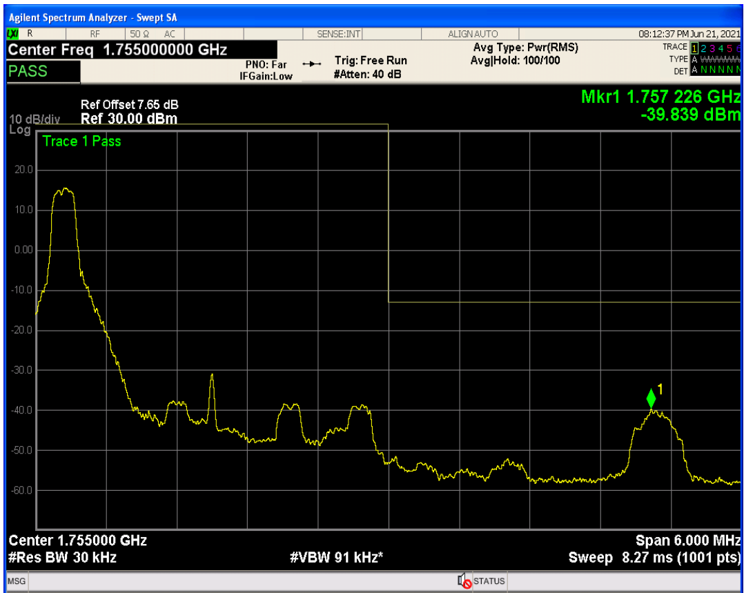
Band4 QAM16 BW=3MHz Channel=19965 RB Size=15 Position=#0
