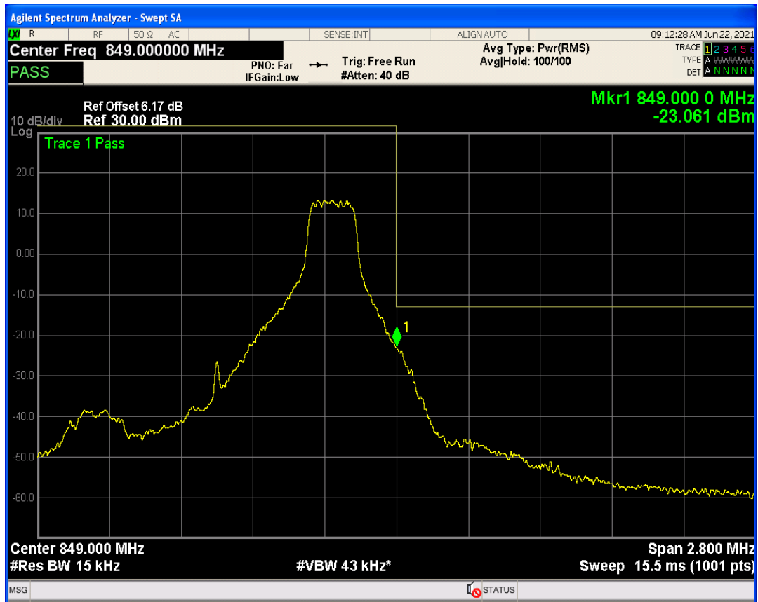
Band5 QPSK BW=1.4MHz Channel=20643 RB Size=6 Position=#0
