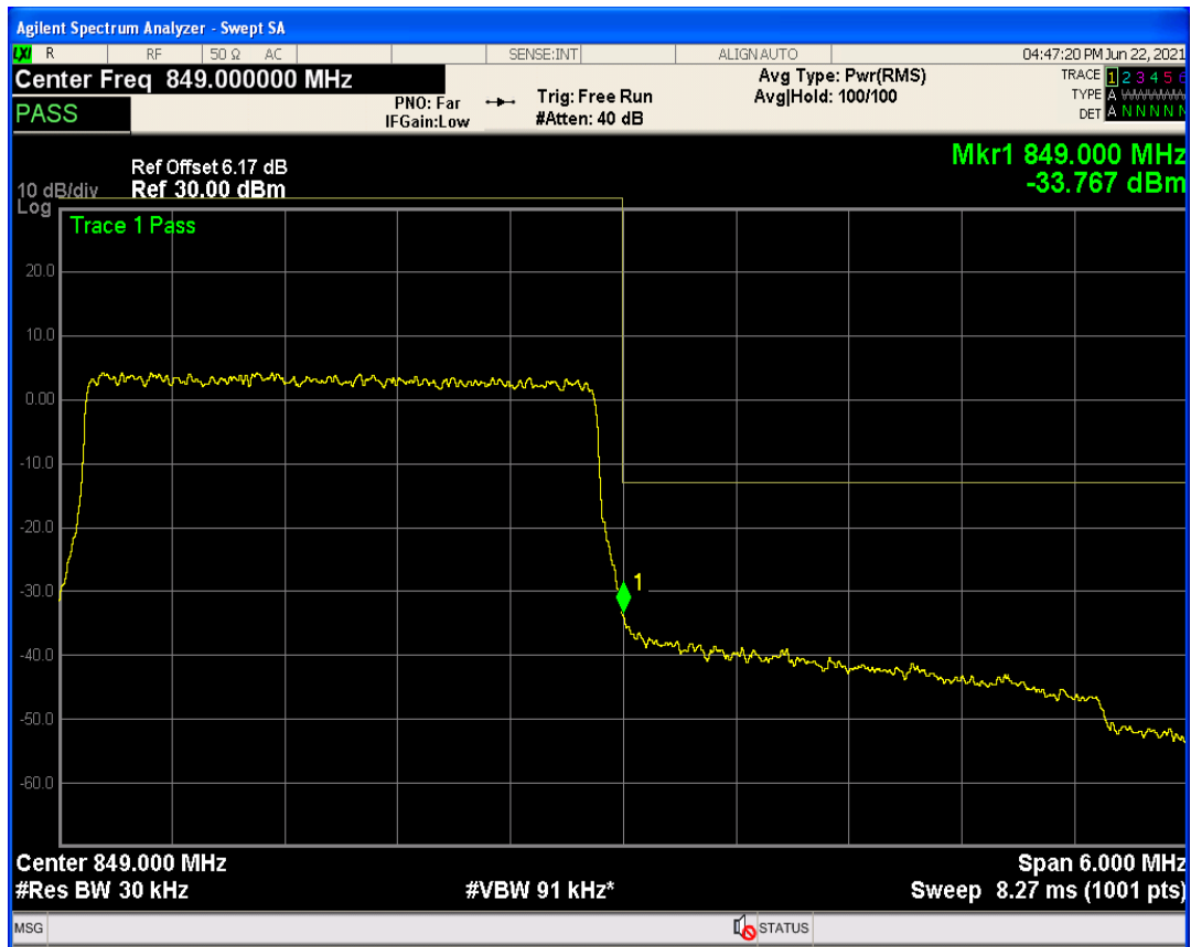
Band26b QPSK BW=3MHz Channel=27025 RB Size=1 Position=#Max
