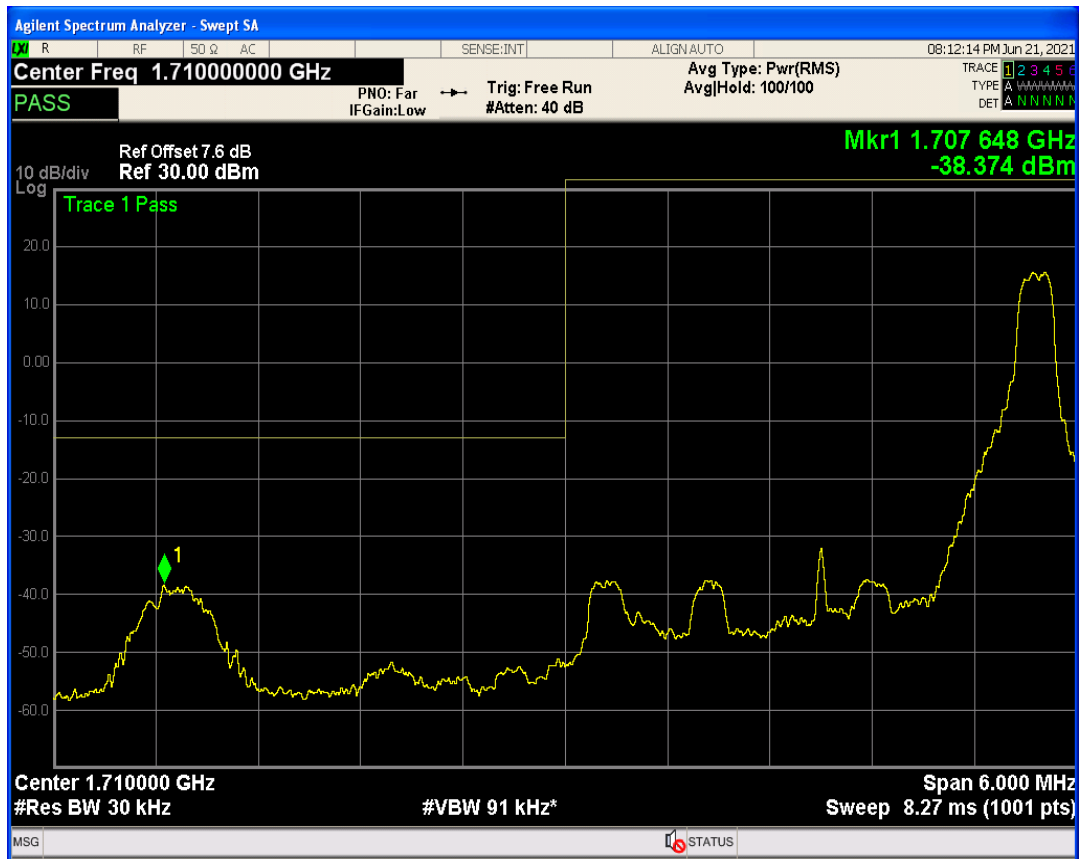
Band4 QAM16 BW=3MHz Channel=19965 RB Size=1 Position=#0
