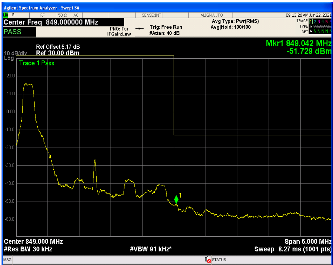
Band5 QAM16 BW=3MHz Channel=20415 RB Size=15 Position=#0
