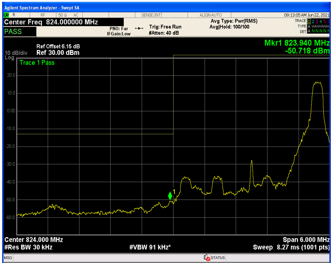
Band5 QPSK BW=3MHz Channel=20415 RB Size=15 Position=#0
