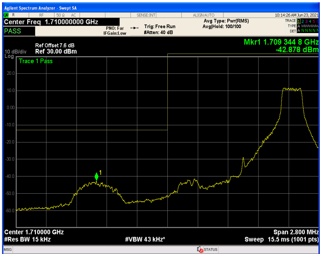
Band66 QPSK BW=1.4MHz Channel=132665 RB Size=1 Position=#0
