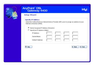
4 Select the Specify an IP Address (Static) option, enter the IP Address, Subnet Mask, and Default Gateway information in the fields provided, then click Next.
