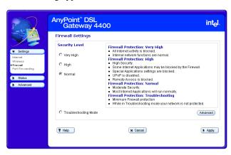
3 Select a security level from the main screen, specify intrusion detection settings or specify IP addresses to be excluded from the firewall detection system from the Advanced screen. You can also allow your service provider to troubleshoot your network directly by clicking the **Troubleshooting mode** option.
