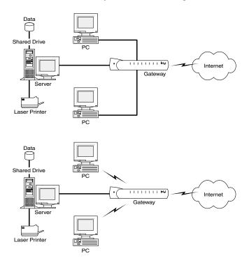
The Intel AnyPoint DSL Gateway 4400 connects directly to a DSL (Digital Subscriber Line) using the built-in DSL modem. Using the gateway and its built-in DSL modem together enables powerful Internet access on a home or small-business network.
