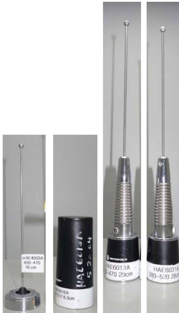
UHF2 Antenna kit numbers, from left to right HAE4003A, HAE6016A, HAE6013A, HAE6031A
