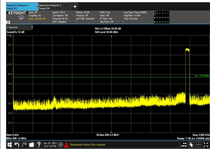
Spurious Emissions at Antenna Terminal QPSK 60MHz B.W.; 2660.0MHz, 60kHz
