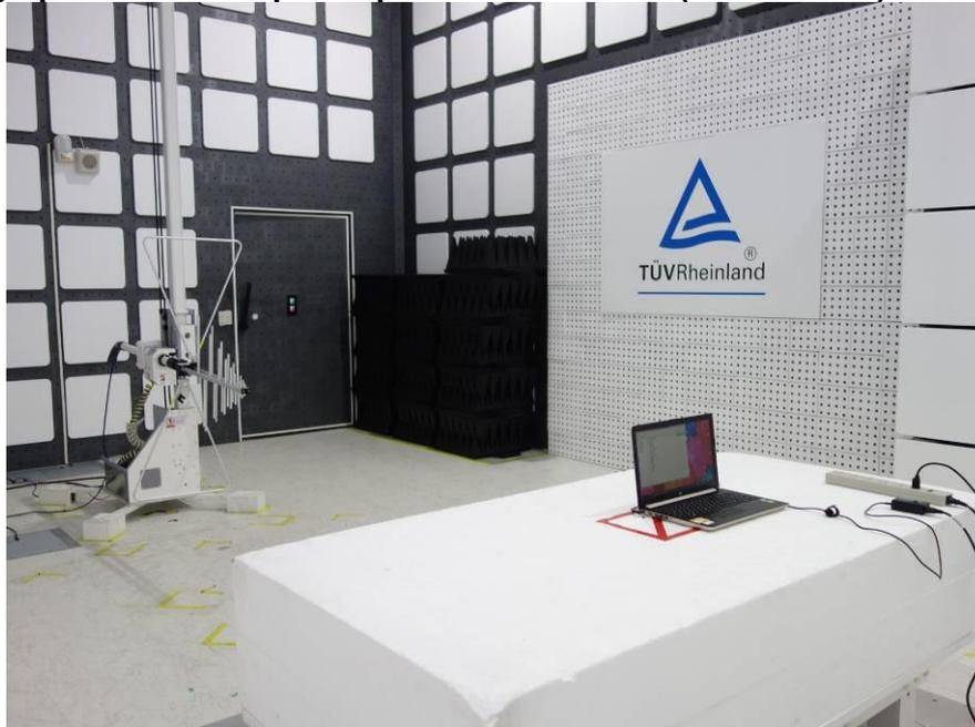
**Photograph 4: Test Setup for Spurious Emissions (Back View 2)**
