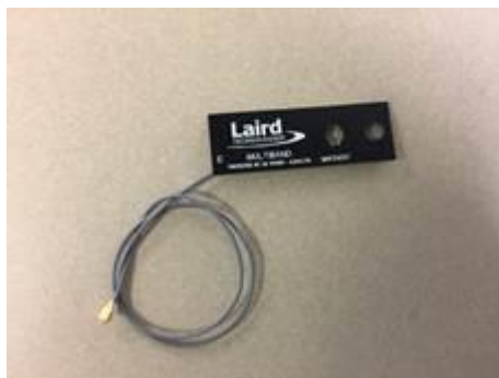
Wifi Module Antenna: It is installed on the interior of the plastic enclosure.
