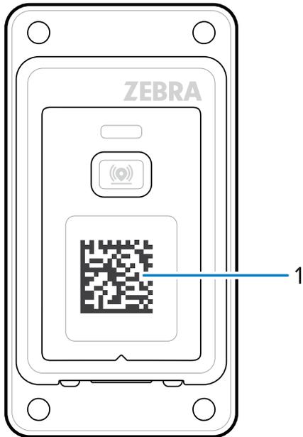
The Status LED blinks blue, indicating that the RS2100 is attempting to establish a connection with the device. When a connection is established, the Status LED turns off, and the RS2100 emits a single string of low/high beeps.
